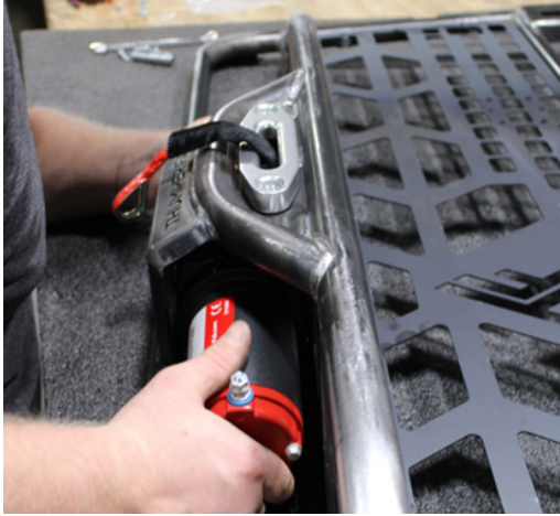
FIG 3 - Thread Winch Cable through Fairlead
