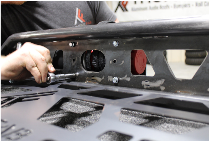
FIG 4 - Fasten Winch to Winch Base Plate with 10mm Socket
