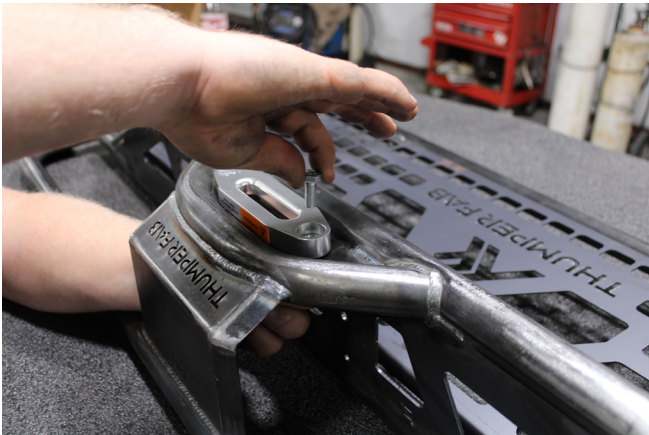
Fig 2 - Fasten fairlead to Headache Rack
