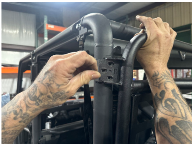
FIG 6 - Fasten Headache Rack Bolts
