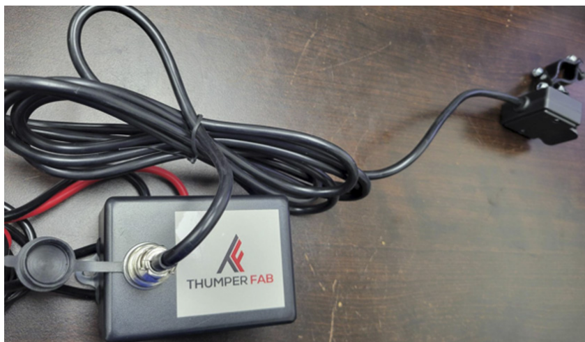
FIG 10 - Tighten switch harness to contactor box
