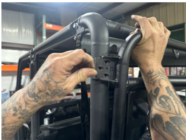
FIG 6 - Fasten Headache Rack Bolts
