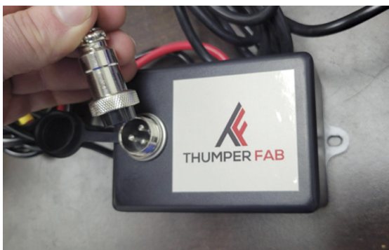
FIG 9 - Plug manual switch harness into winch contactor box
