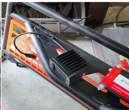
FIG 14 - Zip Tie Cube Light wire pigtail to Headache Rack
