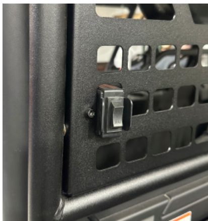
FIG 7 - Fasten switch to accent panel
