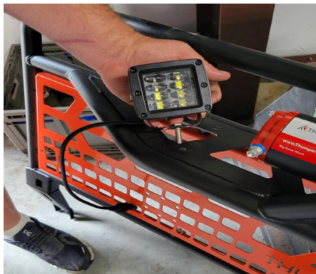
FIG 13 - Fasten cube light to Headache Rack
