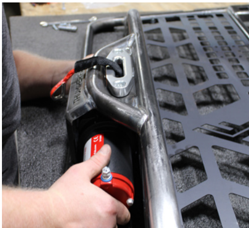
FIG 3 - Thread Winch Cable through Fairlead
