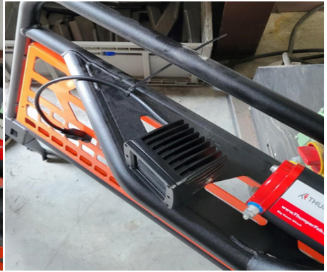
FIG 12 - Zip Tie Cube Light wire pigtail to Headache Rack
