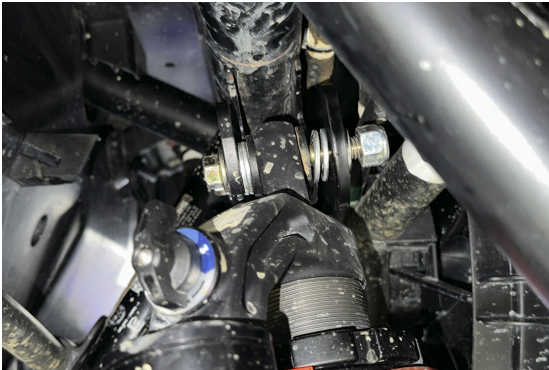
FIG 9 - Mount Shock and tighten hardware, starting with shock bolts first using 18mm Socket and Wrench
