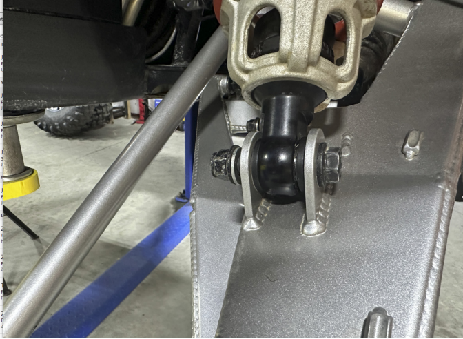
FIG 17 - Mount shock to Upper Control Arm using 18mm Socket and Wrench
