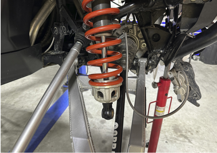
FIG 13 - Install Axles, mount Front Lower Control Arms using OEM Hardware
