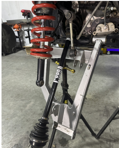
FIG 24 - Mount Rear Lower Control Arm using Factory Hardware
