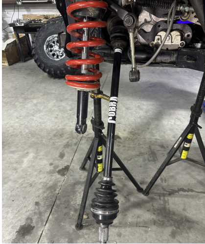
FIG 23 - Reinstall Rear shocks to frame mount, install axle into differential
