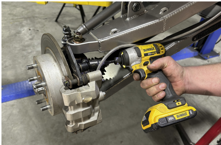
FIG 21 - Fasten Brake Caliper to Knuckle using a 15mm Socket
