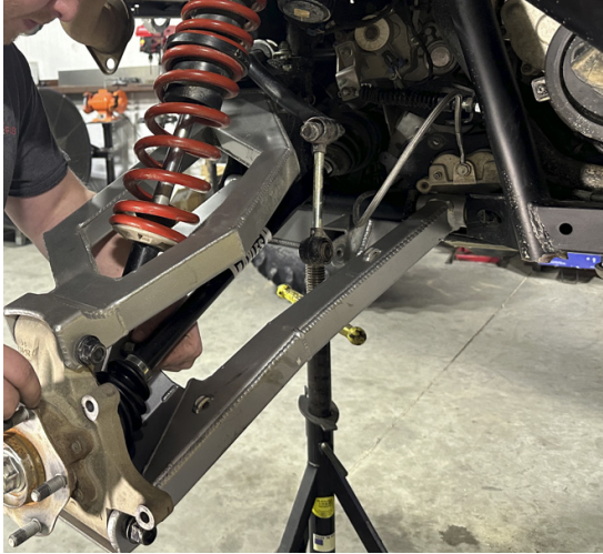
FIG 25 - Reinstall Knuckle, Tighten Axle Nut using 30mm Socket, and mount Upper Arm using OEM Hardware
