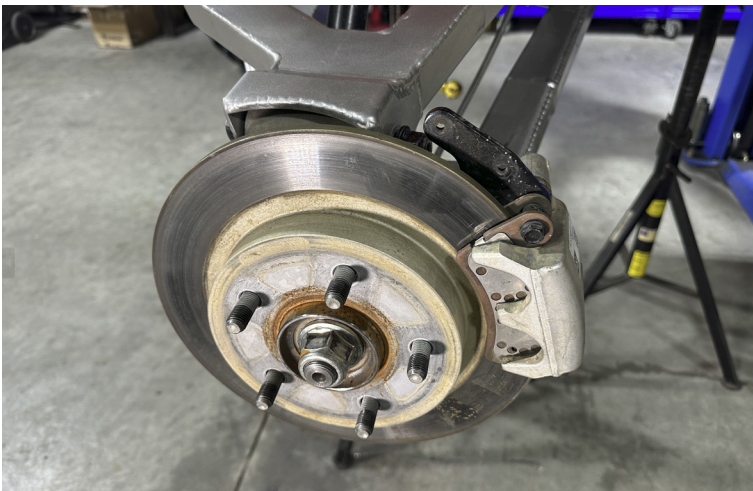
FIG 28 - Reinstall Brake Rotor and Caliper using a 15mm Socket
