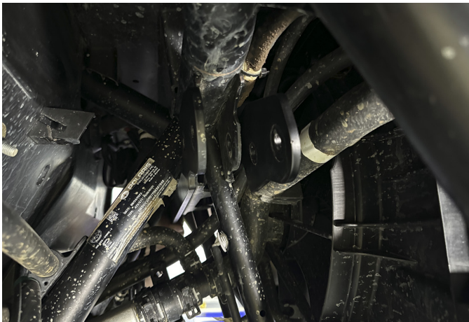
FIG 7 - Place Shock Relocation Brackets into position
