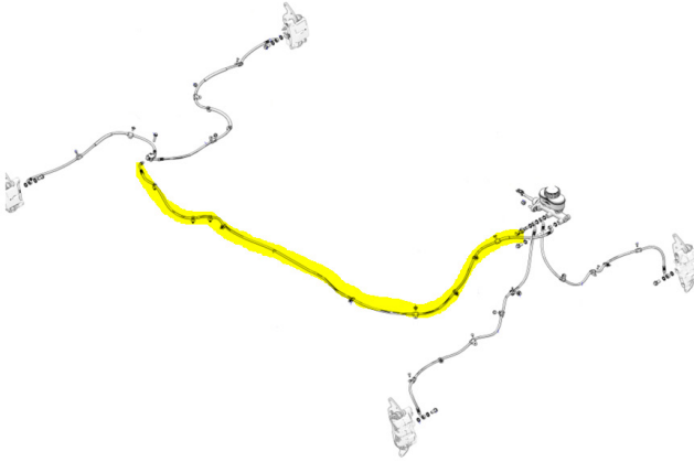
FIG 10 - Replace Brake Lines using provided kit
