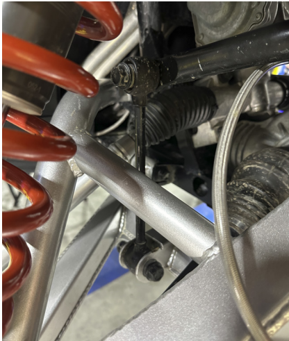
FIG 18 - Mount sway bar link to lower control arm using 18mm Socket and Wrench
