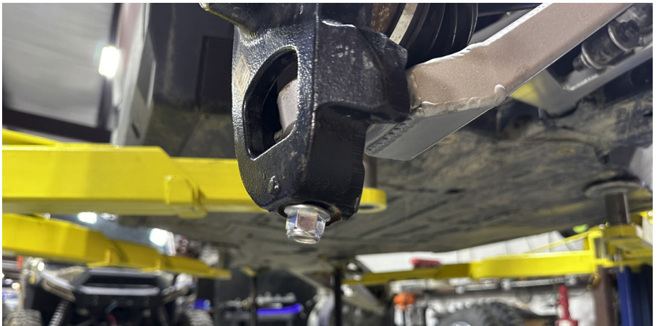
FIG 14 - Mount Knuckles to Lower Ball Joints using 18mm Socket
