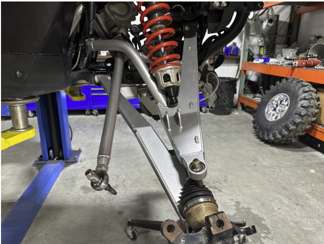
FIG 15 - Mount Front Upper Control Arms using OEM Hardware
