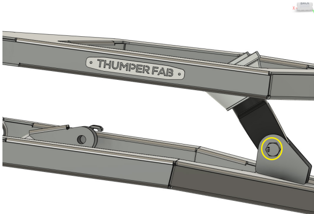
FIG 26 - Fasten Shock to Lower Control Arm using 18mm Socket and wrench
