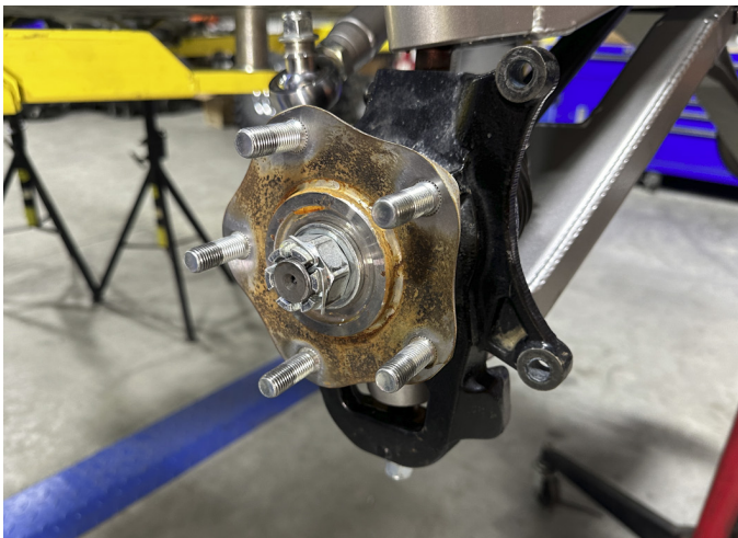
FIG 20 - Install Hub, tighten Axle nut using 30mm Socket
