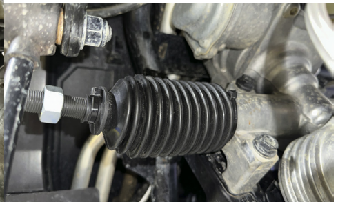
FIG 5 - Fasten Boot to steering rack and Inner Tie Rod using Zip Ties
