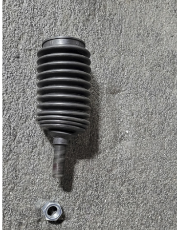
FIG 3 - Slide Inner Tie Rod end through steering rack boot and reinstall jam nut
