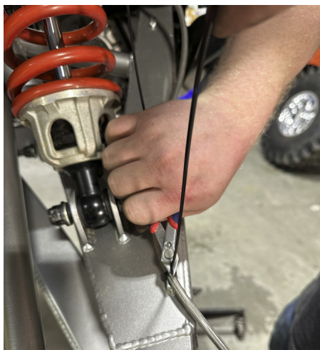
FIG 22 - Zip Tie brake lines to Upper Control Arms
