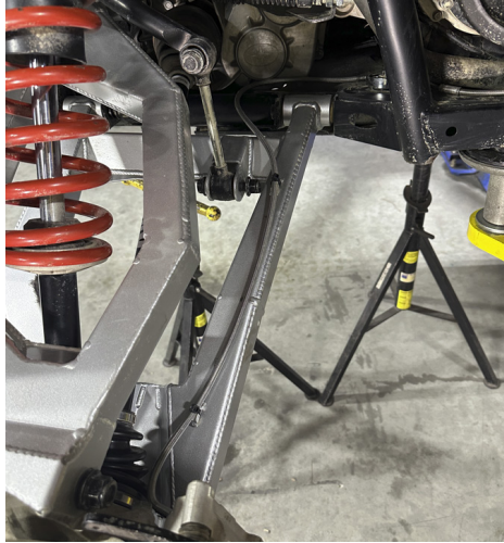
FIG 29 - Fasten Brake Lines to Lower Arm
