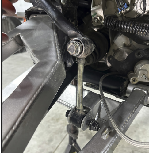
FIG 27 - Fasten Sway Bar Link to Lower Control Arm using an 18mm Socket and Wrench
