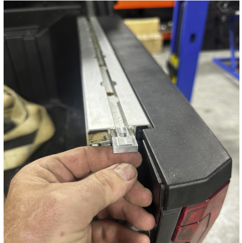
FIG 1 & FIG 2 - Remove bed plug and insert Lock and Ride Max Fasteners into Bed Rail
