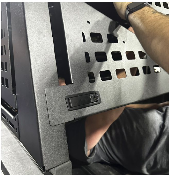
FIG 22 - Mount Compression Latches to the Rear Hatch
