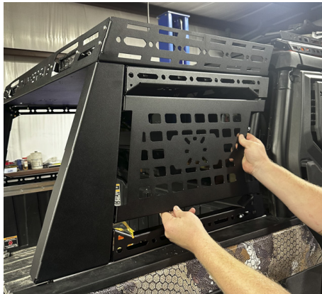
FIG 13 - Mount Side Panels to Bed Rack
