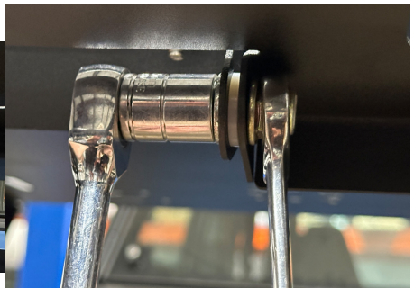
FIG 17 & FIG 18 - Mount Rear Hatch to Hinges
