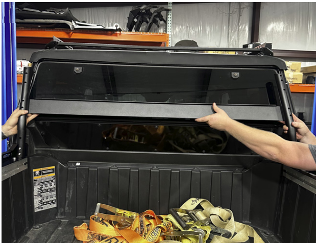
FIG 7 - Mount Forward Brace to Front Pillars
