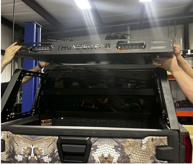
FIG 12 - Mount Top Basket to Top Rails and Rear Pillars
