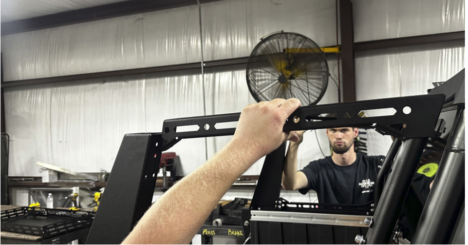
FIG 8 - Mount Top Rails to Front and Rear Pillars
