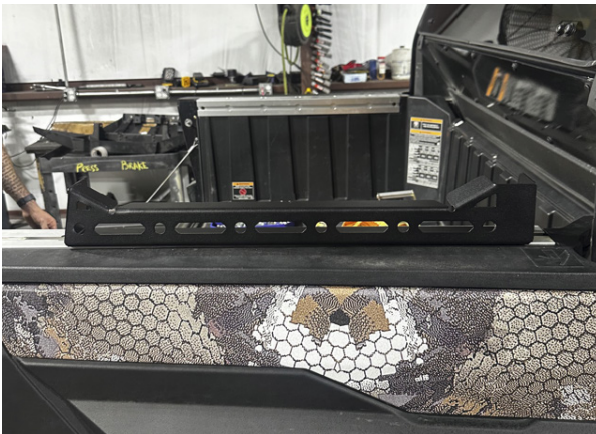
FIG 3 - Loosley Fasten Bottom Rails to Bed Rail
