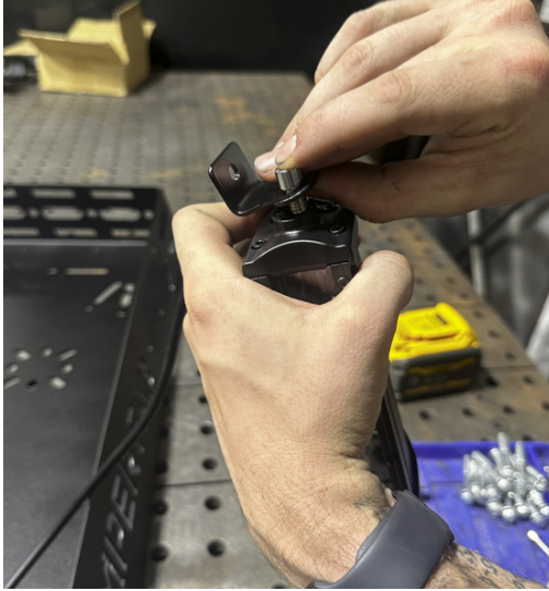
FIG 10 - Mount Light Bar Brackets to Light Bars (OPTIONAL)
