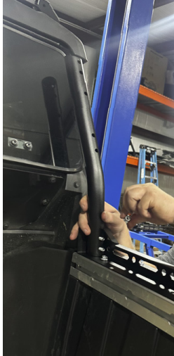
FIG 6 - Mount Front Pillars to Bottom Rails
