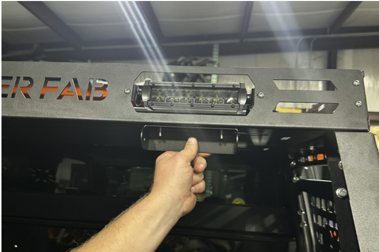
FIG 16 - Mount Hinges to Top Basket
