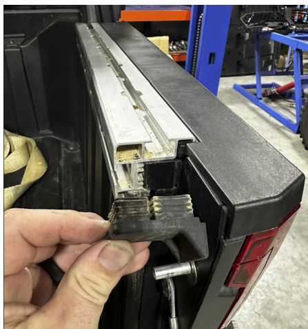
FIG 1 & FIG 2 - Remove bed plug and insert Lock and Ride Max Fasteners into Bed Rail
