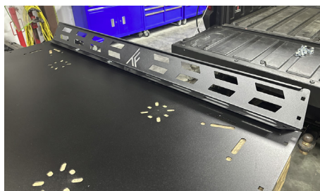
FIG 3 & FIG 4 - Loosley Fasten Basket Front to Basket Base
