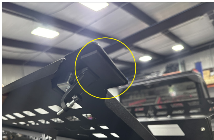
FIG 20 - Apply Foam to Rear Hatch
