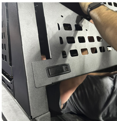
FIG 19 - Mount Compression Latches to the Rear Hatch
