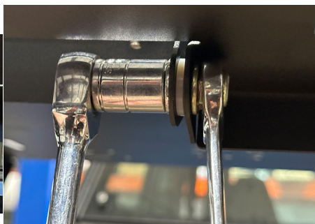
FIG 14 & FIG 15 - Mount Rear Hatch to Hinges
