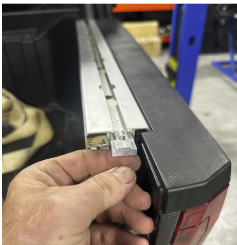
FIG 1 & FIG 2 - Remove bed plug and insert Lock and Ride Max Fasteners into Bed Rail
