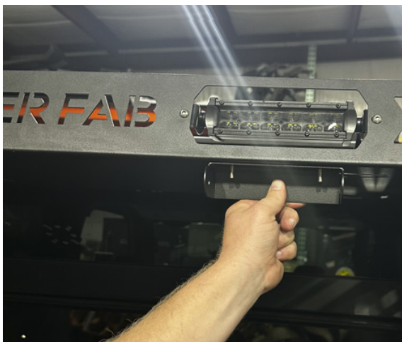
FIG 13 - Mount Hinges to Basket
