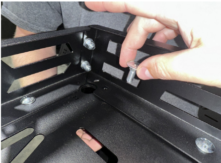
FIG 6 & FIG 7 - Fasten Side Panels to Basket
