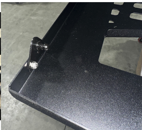
FIG 16 & FIG 17 - Mount Strut Mount Bracket to Side Panels and Rear Hatch
