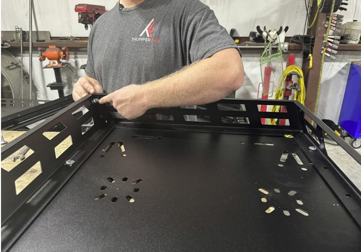
FIG 5 - Mount Basket Side Rails (DR & PA) to Basket Front and Rear Rails
