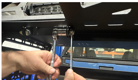
FIG 14 & FIG 15 - Mount Rear Hatch to Hinges
