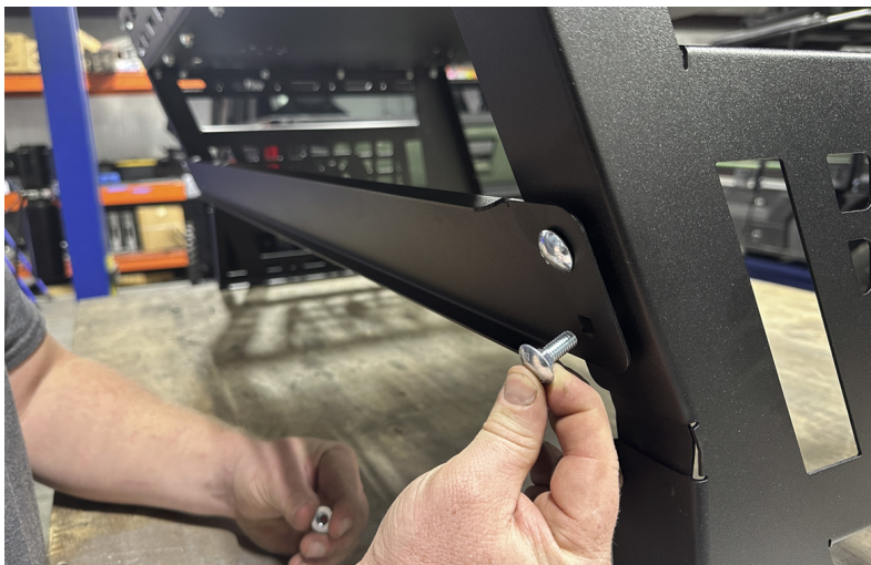
FIG 8 - Mount Front Brace to the Side Panels
