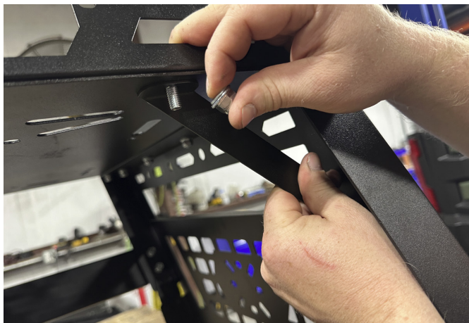
FIG 9 - Fasten Sway Supports to Basket Bottom and Side Panels
