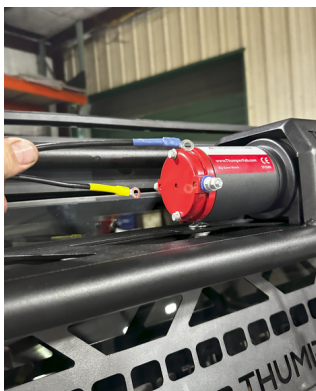
FIG 28 - Connect Winch Control Box to the Winch
