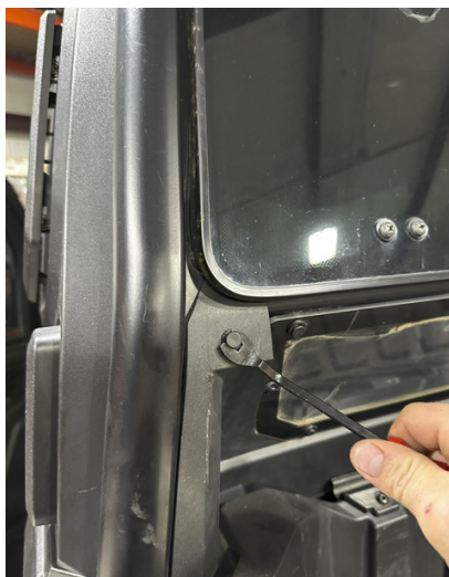
FIG 8 - Remove Outer Panel Clips
