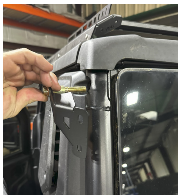
FIG 23 & FIG 24 - Fasten Upper Mounts to Vehicle. Tighten all Hardware
