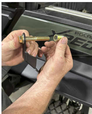
FIG 23 & FIG 24 - Fasten Upper Mounts to Vehicle. Tighten all Hardware
