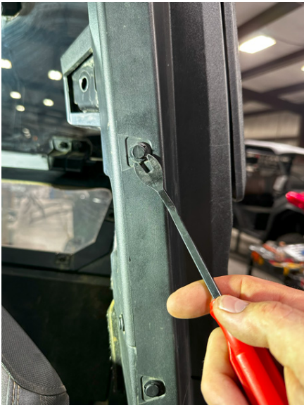
FIG 5 & FIG 6 - Remove Panel Clips and Inside Rear Panel
