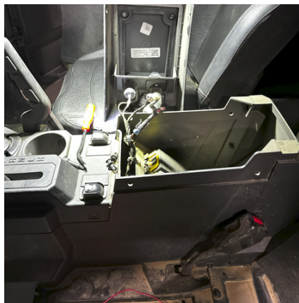
FIG 29 & FIG 30 - Connect Red (Ignition) wire to Key On Power
