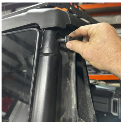
FIG 9 - Remove OEM Roll Cage Bolts
