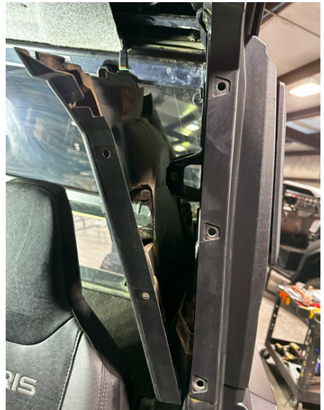
FIG 5 & FIG 6 - Remove Panel Clips and Inside Rear Panel
