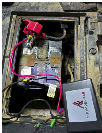
FIG 26 - Connect Winch Control Box to the Battery
