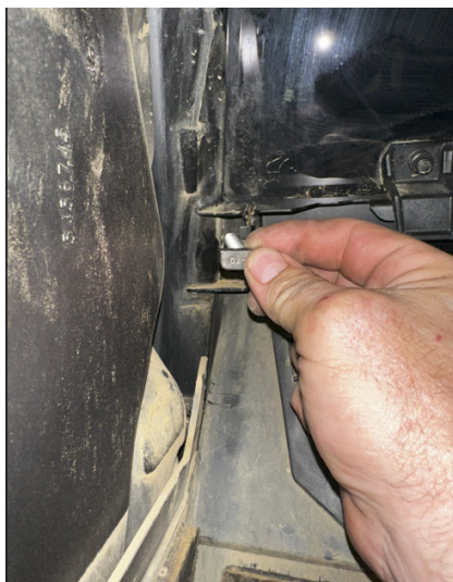
FIG 19 - Insert M8x25mm T-Slot Stud through the vehicle
