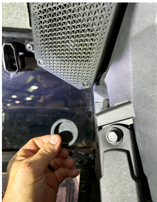
FIG 1 - Remove Panel Plug
