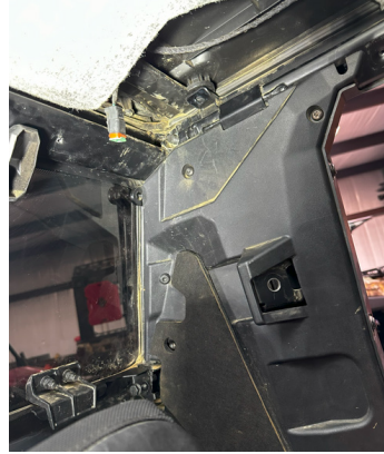
FIG 3 & FIG 4 - Remove Rear Speakers
