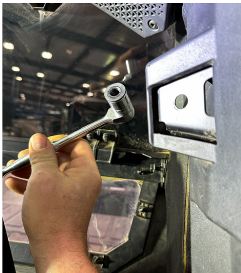
FIG 2 - Unfasten Seat Belt from Vehicle Frame
