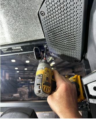
FIG 3 & FIG 4 - Remove Rear Speakers
