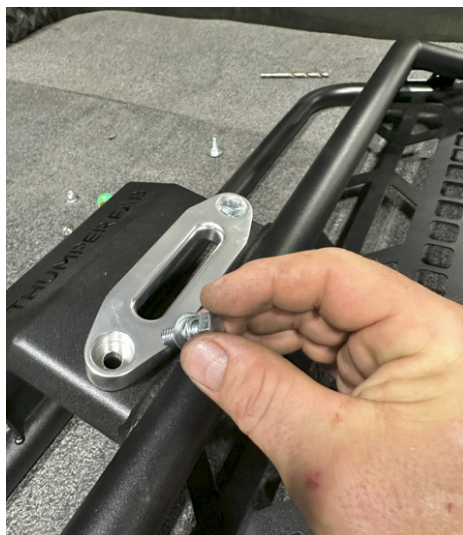
FIG 16 - Fasten Fairlead to the Headache Rack Frame
