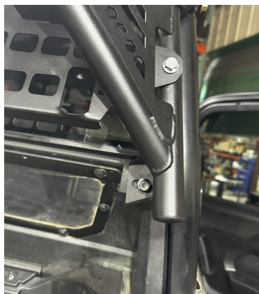
FIG 20 & FIG 21 - Loosley fasten Headache rack to Vehicle
