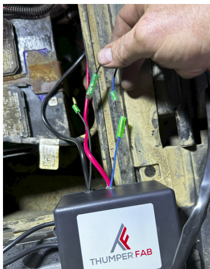
FIG 27 - Connect Winch Control Switch
