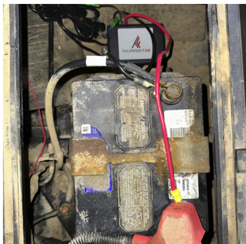
FIG 32 - Fasten Winch Control Module
