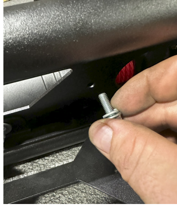
FIG 17 & FIG 18 - Fasten Winch to the Headache Rack Assembly
