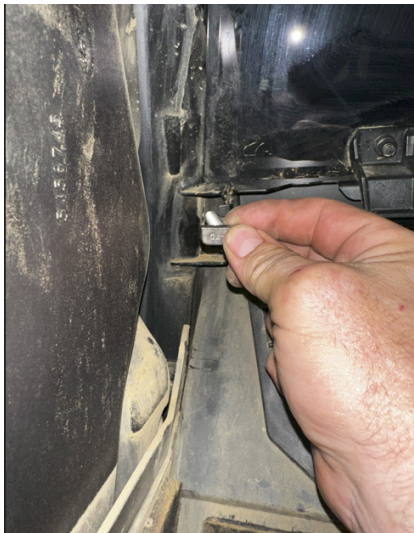
FIG 19 - Insert M8x25mm T-Slot Stud through the vehicle
