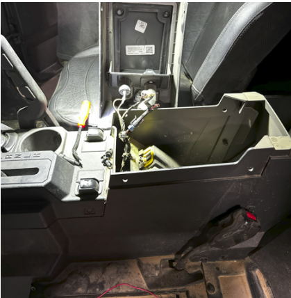
FIG 31 & FIG 32 - Connect Red (Ignition) wire to Key On Power
