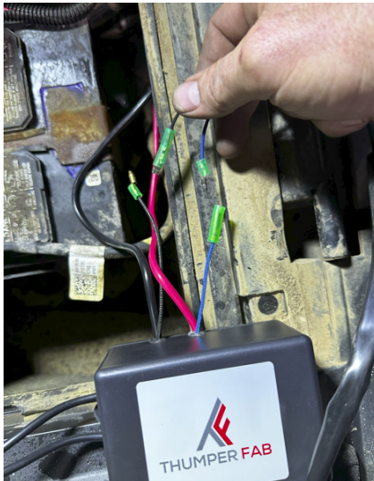
FIG 29 - Connect Winch Control Switch
