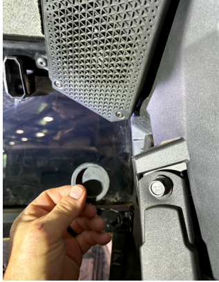
FIG 1 - Remove Panel Plug
