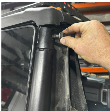
FIG 9 - Remove OEM Roll Cage Bolts
