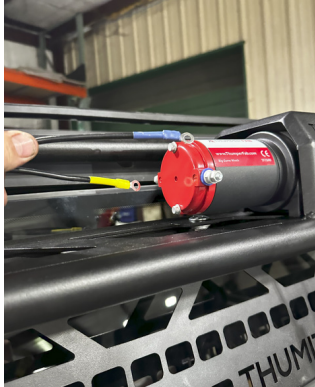
FIG 30 - Connect Winch Control Box to the Winch
