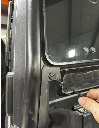
FIG 8 - Remove Outer Panel Clips
