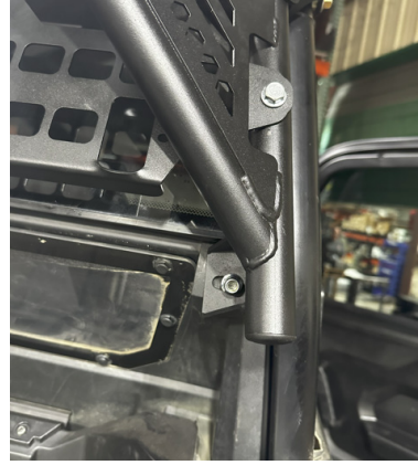
FIG 20 & FIG 21 - Loosely fasten Headache rack to Vehicle
