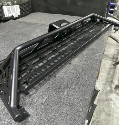
FIG 11 & FIG 12 - Install and fasten Rear Panel to Headache Rack Frame
