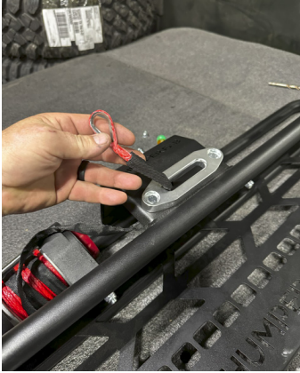
FIG 17 & FIG 18 - Fasten Winch to the Headache Rack Assembly
