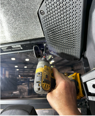
FIG 3 & FIG 4 - Remove Rear Speakers
