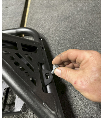
FIG 11 & FIG 12 - Install and fasten Rear Panel to Headache Rack Frame
