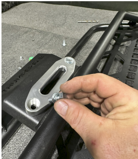
FIG 16 - Fasten Fairlead to the Headache Rack Frame
