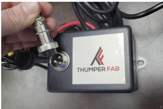
FIG 26 - Plug manual switch harness into winch contactor box
