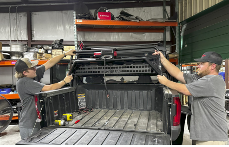
FIG 20 & FIG 21 - Loosely fasten Headache rack to Vehicle
