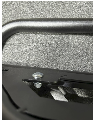
FIG 13 - Fasten top of Rear Panel to the Headache Rack Frame
