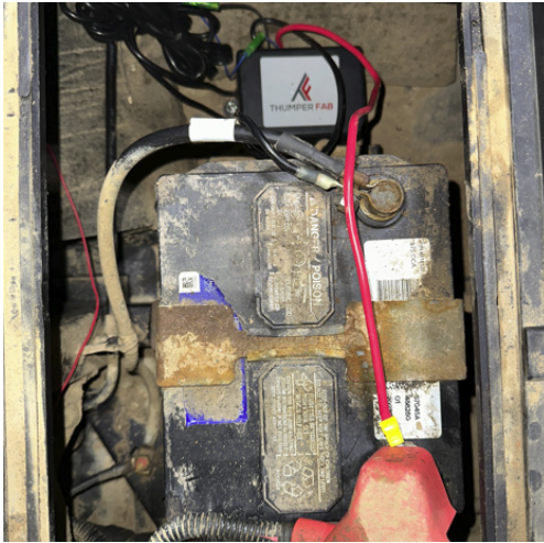
FIG 34 - Fasten Winch Control Module
