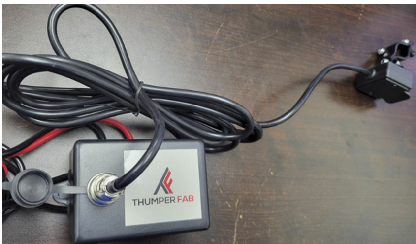
FIG 27 - Tighten switch harness to contactor box
