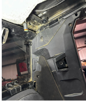
FIG 3 & FIG 4 - Remove Rear Speakers
