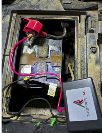
FIG 28 - Connect Winch Control Box to the Battery
