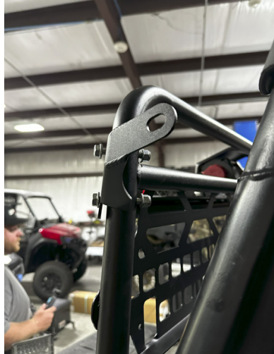
FIG 22 - Fasten Upper Mount Brackets to the Headache Rack Frame
