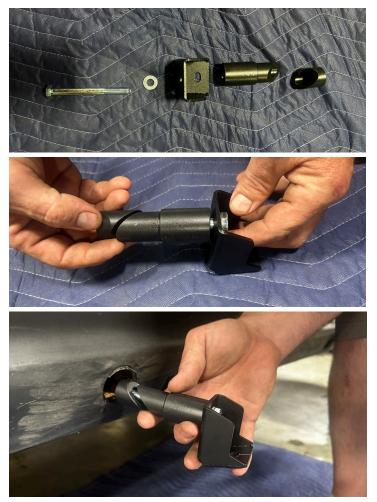
Tighten the M10 bolt just enough to create tension inside the mount tube in the frame, but loose enough so that the mount bracket still swivels. It will be completely tightened after the Nerf Rail Bottom Body has been installed into place.
