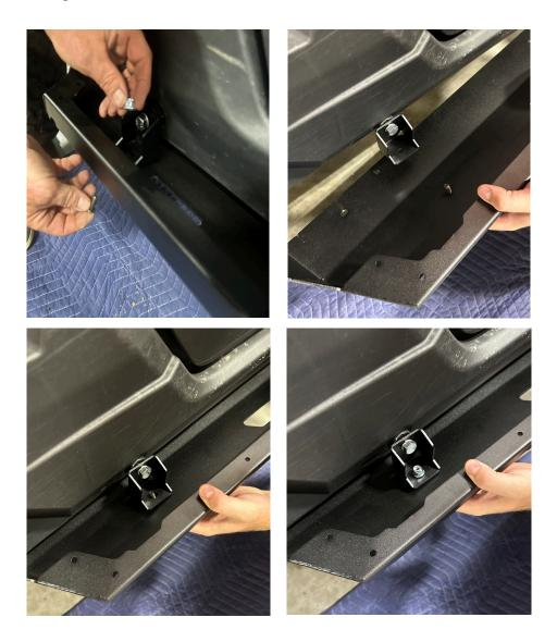
Next, continue fastening the Bottom Body using the M6 x 30mm screws where the OEM Torx screws were previously removed. Tighten these and then move onto tightening all of the M10 and M8 hardware as well.
