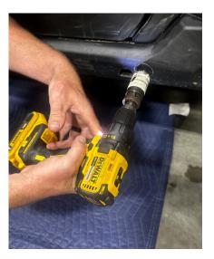
Next, locate the wedge anchor, through hole mounts and threaded wedges, mount brackets, M10 x 100mm bolts, and M10 Split washers. Pre-assemble the wedge anchor/mount brackets sub-assemblies as shown below. Then install them into the previously drilled holes.
