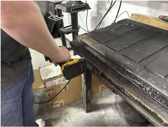
FIG 10 - Reinstall T40 Torx bolts and mount Tailgate back on vehicle
