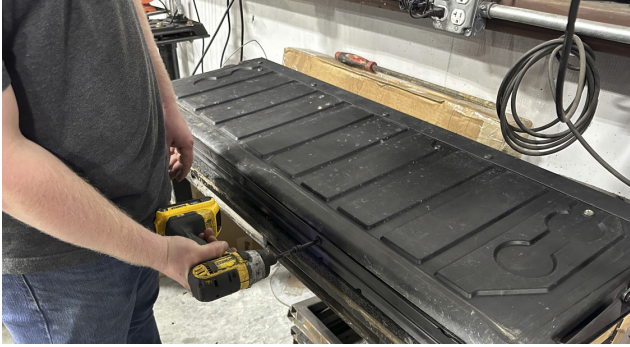
FIG 9 - Remove Drip Lip using a T40 Torx
