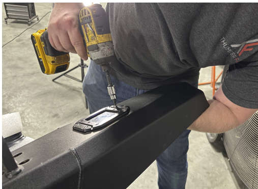
FIG 4 - Mount Cube Lights or Cube Light Covers using 5/32" Allen and 7/16" Wrench
