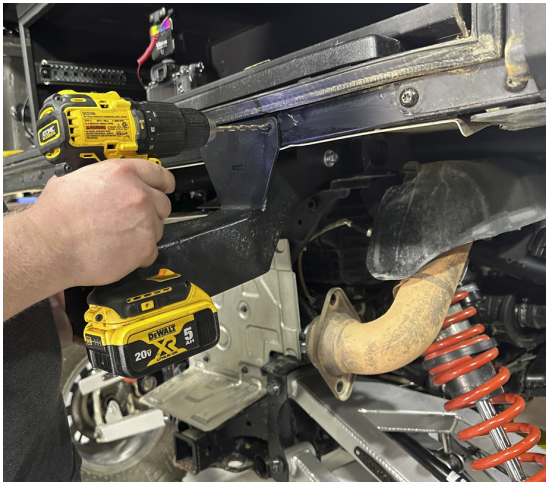
FIG 6 - Use a 1/4" Drill bit to drill pilot holes using Brackets (2&3) as a template
