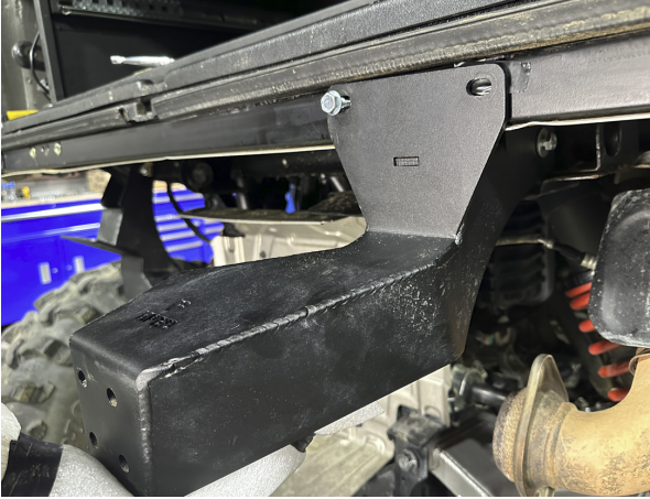
FIG 7 - Use Thread Forming screw to prepare for 5/16" Button Head Screws
