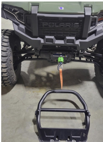
FIG. 3 - Remove the bumper from the vehicle
