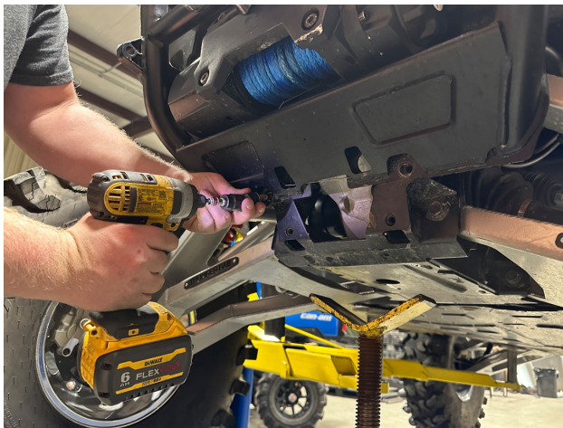
FIG. 1 - Remove Lower Bumper Mounting Bolts using 15mm Socket
