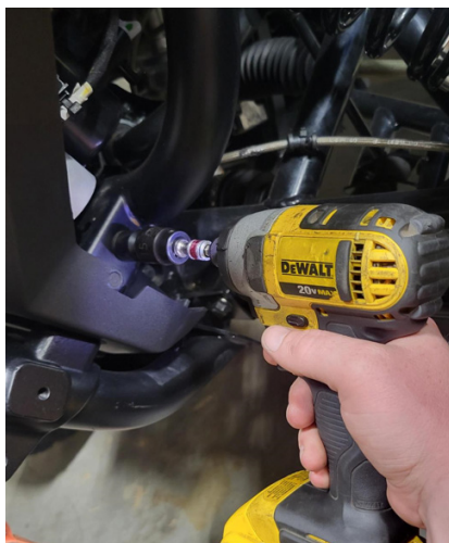
FIG. 2 - Remove Upper Bumper Mounting Bolts using 15mm Socket & Wrench
