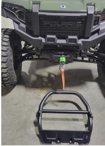
FIG 3 - Remove the bumper from the vehicle
