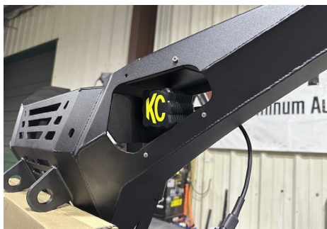
FIG 11 - Mount light mounts, hole covers, and light covers depending on desired appearance. Tighten using 9/64" Allen and 11/32" Wrench
