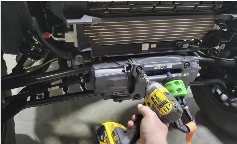
FIG 7 - Remove winch mounting bolts using an 8mm Allen
