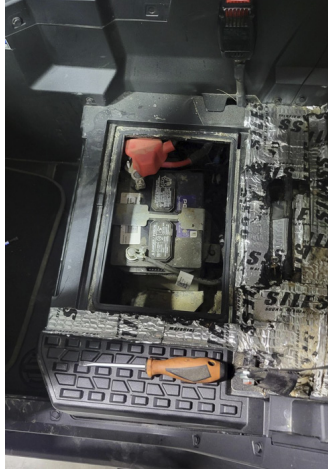
FIG 6 - Disconnect battery using a 10mm Socket and 13mm Wrench
