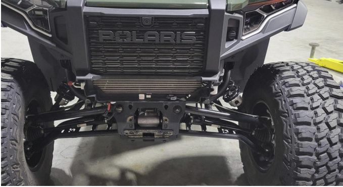
FIG 8 - Remove the winch from the vehicle
