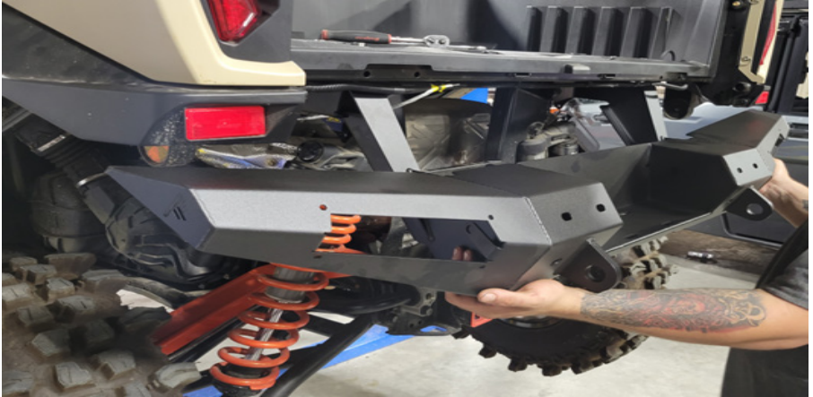
FIG 9 - Slide the main bumper body over the mount brackets
