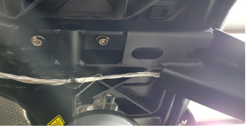
FIG 7 - Start mounting locknuts on OEM studs and 5/16" bolts that go through bed, Do Not Tighten.
