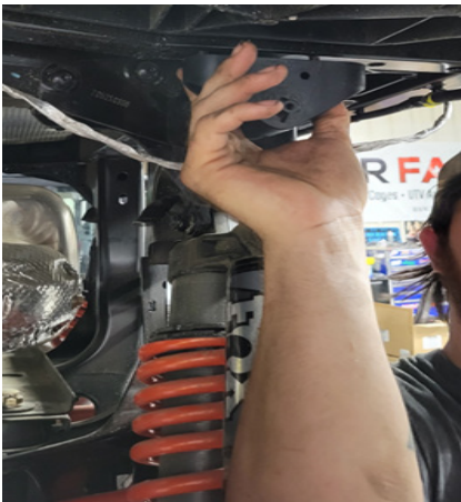
FIG 2 - Use a 15mm Socket to remove OEM Pivot Brackets FIG 3 - Remove O-Ring from Pivot Shaft
