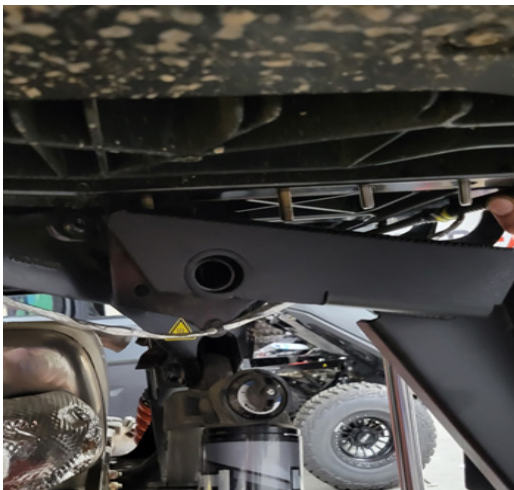
FIG 6 - Slide Brackets over pivot shaft and lower bed so that mounting bolts slide through mount brackets
