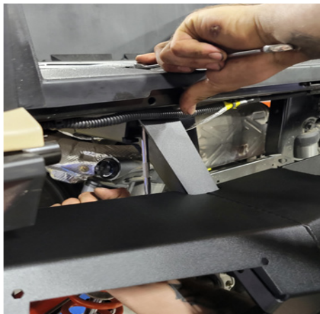
FIG 11 - Tighten mount brackets to unit using 1/2" Socket, 1/2" Wrench, and 15mm Socket
