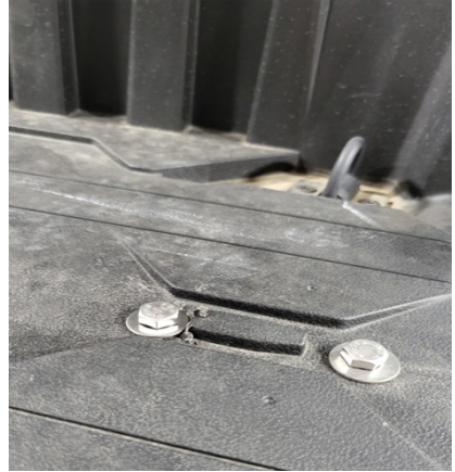
FIG 5 - With surface on bed shaved down, make sure washer sits flat
