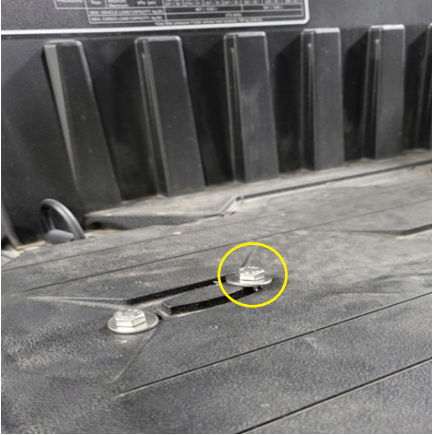
FIG 4 - Place bolts through holes and note area that needs to be shaved
