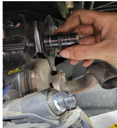
FIG 2 - Use a 15mm Socket to remove OEM Pivot Brackets FIG 3 - Remove O-Ring from Pivot Shaft
