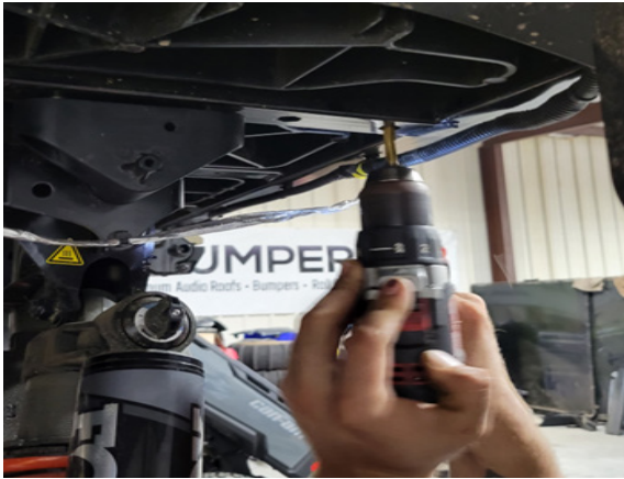
FIG 1 - Remove the tail gate and drill holes using a 5/16" drill bit
