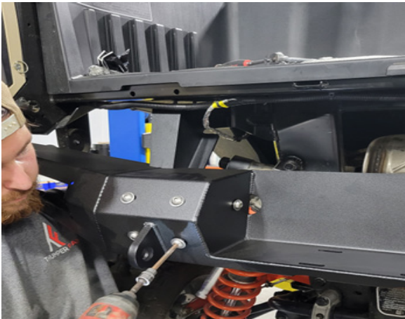
FIG 10 - Fasten Main Bumper Body to Mount Brackets using 7/32" allen and 9/16" Socket
