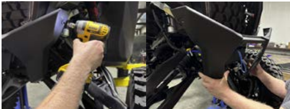
FIG 1 & 2 - Remove Fairlead and Front Plastics
