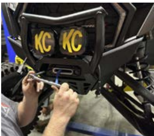
FIG 8 - Mount Outer Fascia and Bumper to Vehicle
