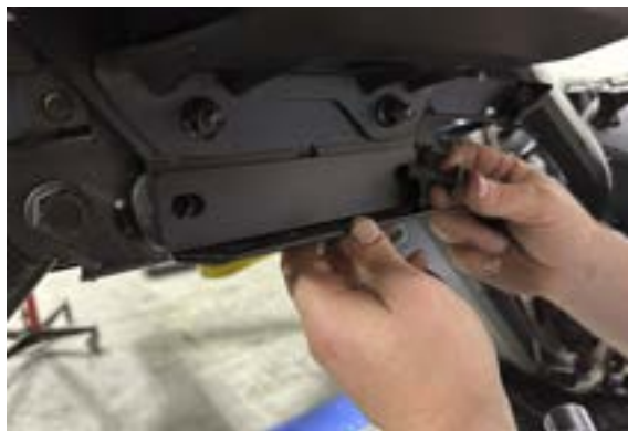
FIG 3 - Loosley Mount Bottom Mount Bracket
