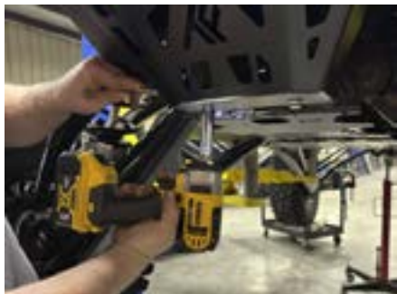
FIG 9 & FIG 10 - Fasten Bumper Body to Bottom Mount Bracket
