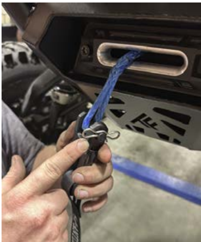
FIG 12 - Reinstall Winch Stop and Winch Hook
