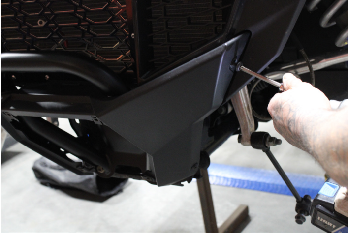
FIG 1 - Remove plastics with T40 Torx
