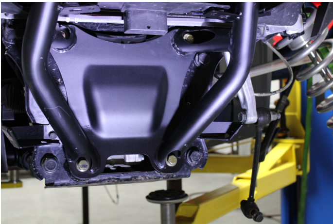
FIG 2 - Remove OEM bumper with 15mm Socket
