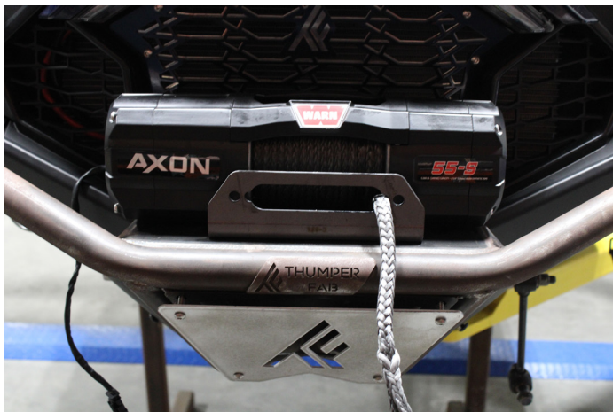
FIG 8 - Mount winch on top of fairlead plate
