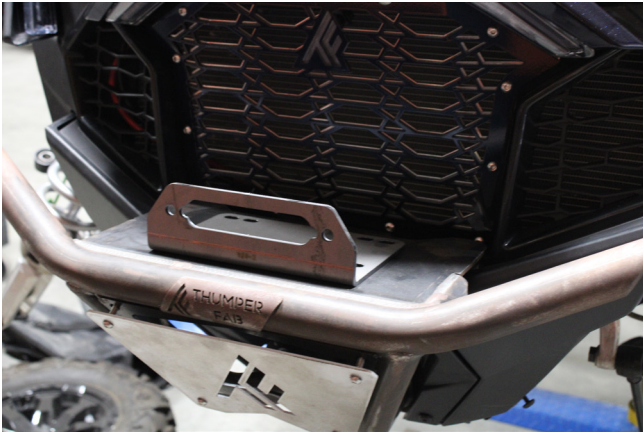
FIG 7 - Place the fairlead on bumper in preparation for winch mounting
