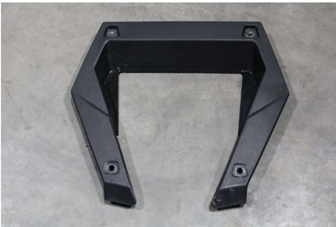
FIG 4 - Trim the plastics using a Sawzall or similar cutting tool
