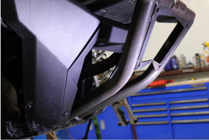
FIG 5 - Remount plastics using factory hardware and T40 Torx
