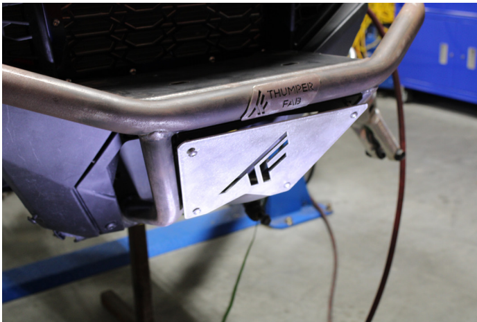
FIG 6 - Mount bumper using 3/16" Allen and 7/16" Socket
