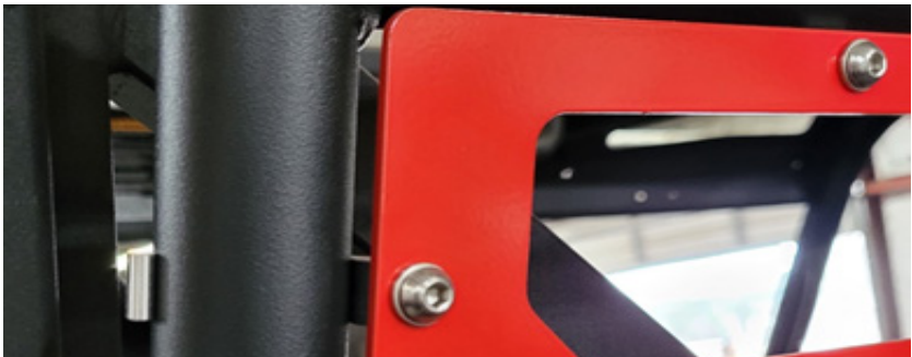
FIG 11 - Install Rear Window Cover 5/32" Allen Wrench
