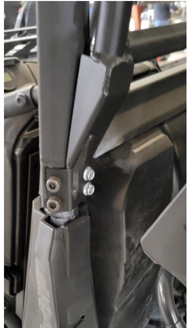
FIG 5 - Thread and tighten lower bolts using 13mm Socket
