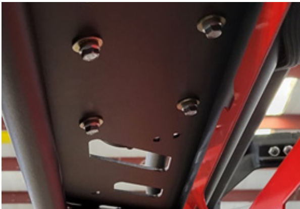
FIG 7 - Install Winch 10mm Socket
