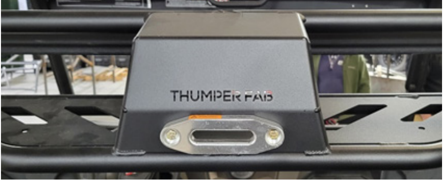
FIG 6 - Install Fairlead using 5/32" Allen Wrench and 7/16" Wrench
