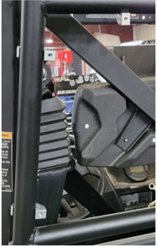
FIG 11 - Install Tubing Clamps
