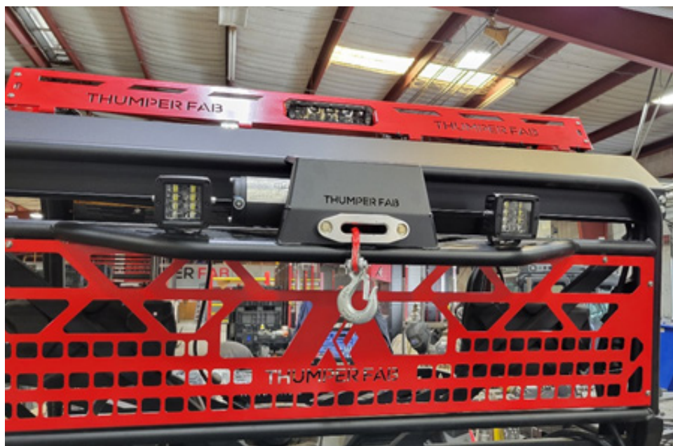
FIG 15 - Install Cube Lights
