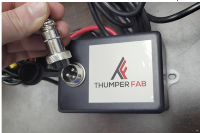
FIG 9 - Plug manual switch harness into winch contactor box
