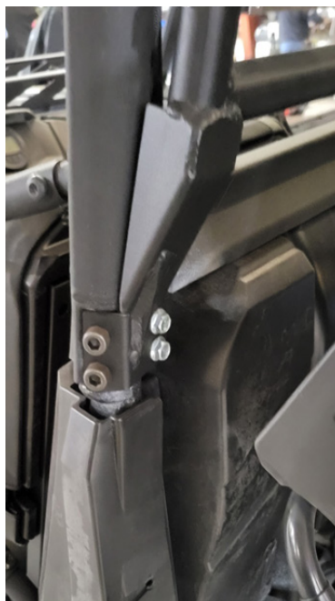
FIG 5 - Thread and tighten lower bolts using 13mm Socket
