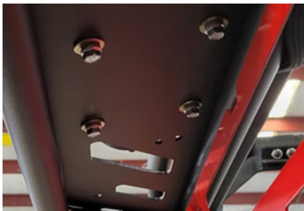
FIG 7 - Install Winch 10mm Socket
