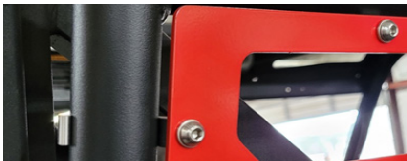
FIG 14 - Install Rear Window Cover 5/32" Allen Wrench
