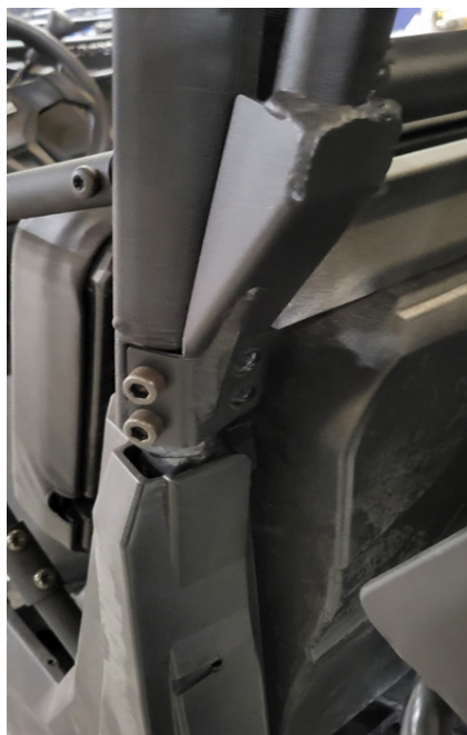
FIG 4 - Thread in M10-1.25 x 60mm socket cap screws using 8mm Allen Wrench
