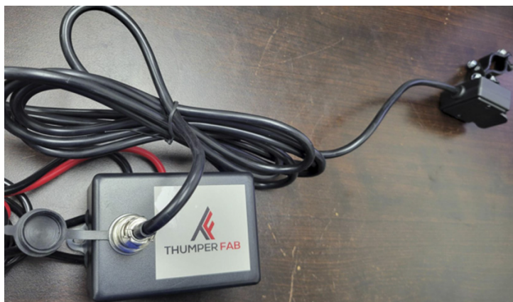
FIG 10 - Tighten switch harness to contactor box
