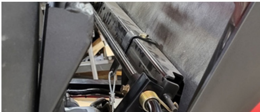
FIG 11 - Install Retention Cable Mount Bracket using 7/16" Socket and 7/16" Wrench
