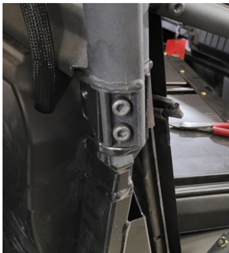
FIG 1 - Remove Lower Stock Bolts (8mm Allen Wrench)
