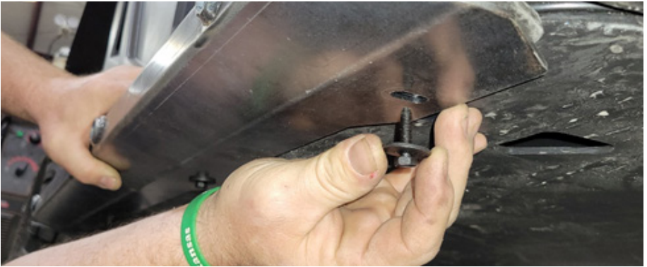
FIG 7 - Tighten up M6-1.0 x 25mm Body Bolts using T-30 Torx Bit
