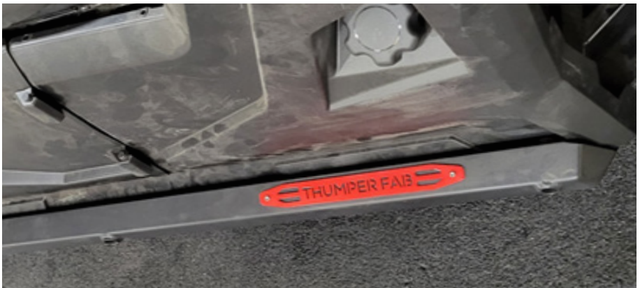
FIG 8 - Install Accent Panel using 9/64" Allen Wrench.
