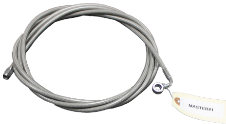
Master 1: From master cylinder to rear
