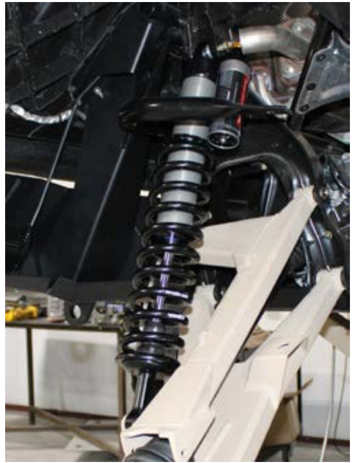
Rear Shock: Reservoir position faces toward front of vehicle
