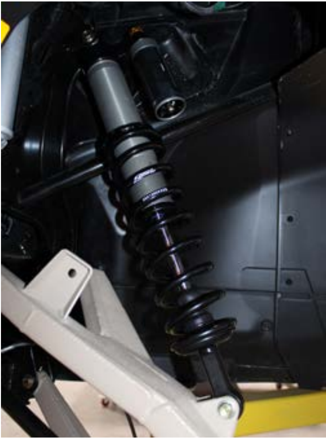
Front Shock: Reservoir position faces outboard of vehicle
