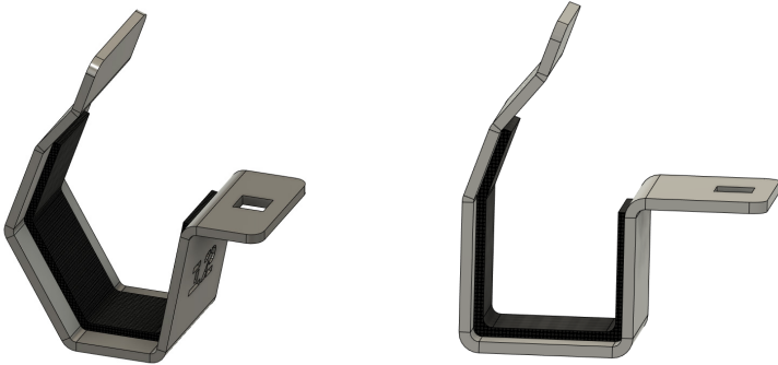
FIG 4 - Apply Foam to Lower Bull Bar Mount Brackets
