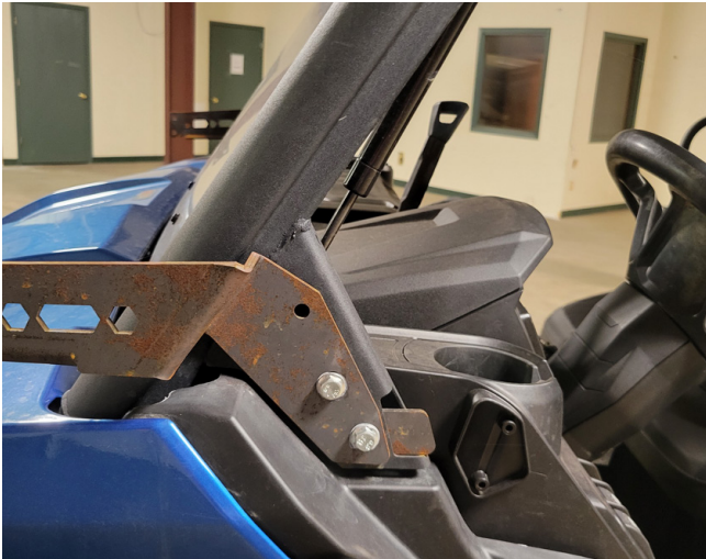
FIG 3 - Mount Rear Mount Brackets using a 13mm Socket
