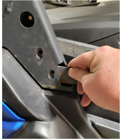
FIG 1 & FIG 2 - Insert Roll Cage Brackets into Roll Cage
