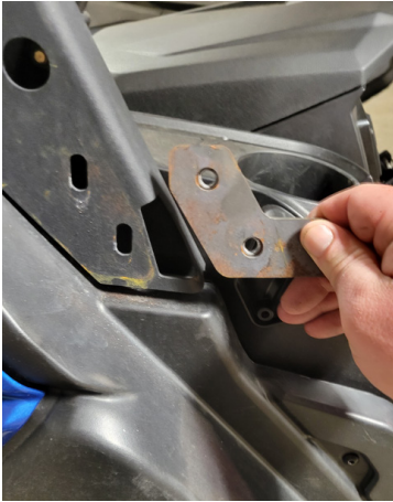
FIG 1 & FIG 2 - Insert Roll Cage Brackets into Roll Cage
