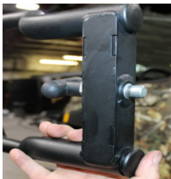
FIG 21 - Install Plastic Tubing Plugs (O)
