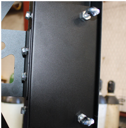
FIG 18 - Loosley install Mount Hinge (14) using 13mm Socket and 13mm Wrench
