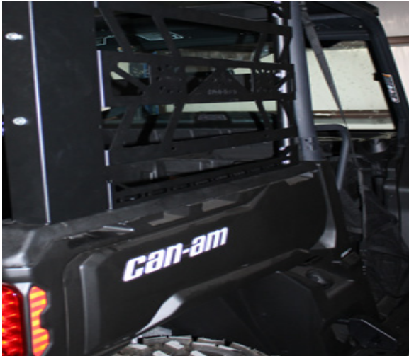
FIG 3 - Put Loosely Assembled side Rails on Bed
