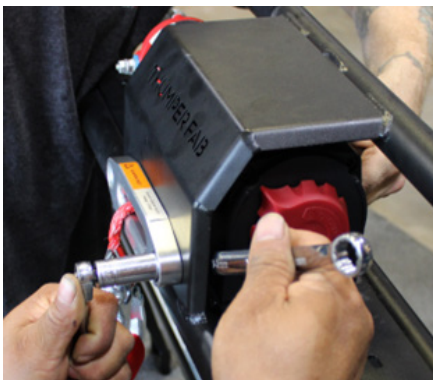
FIG 4 - Fasten Fairlead to Winch Cover Plate
