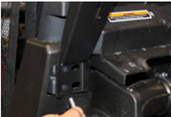
FIG 8 - Fully tighten Flange Bolts (B) using 13mm Socket and Ratchet
