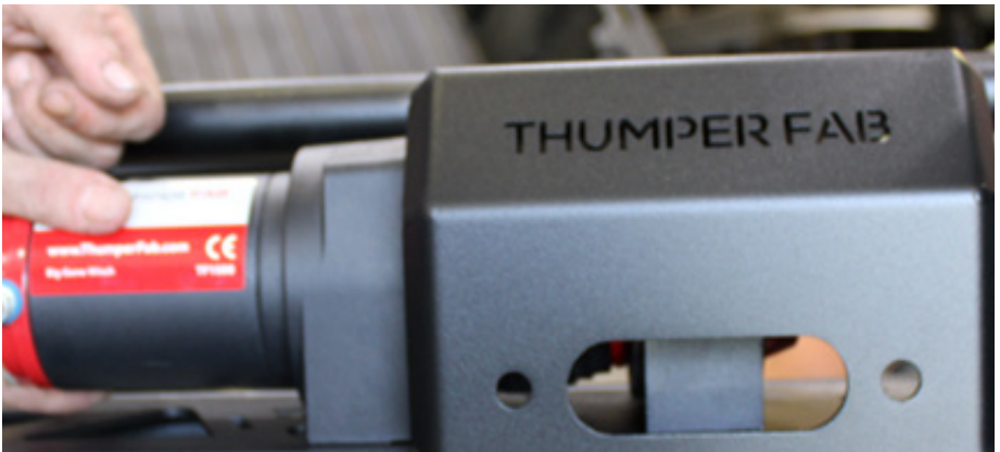
FIG 2 - Slide Winch under Winch Cover Plate
