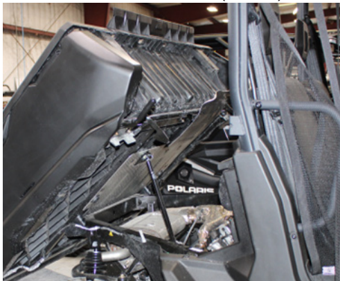
FIG 6 - Raise Dump Bed to Fully Open Position
