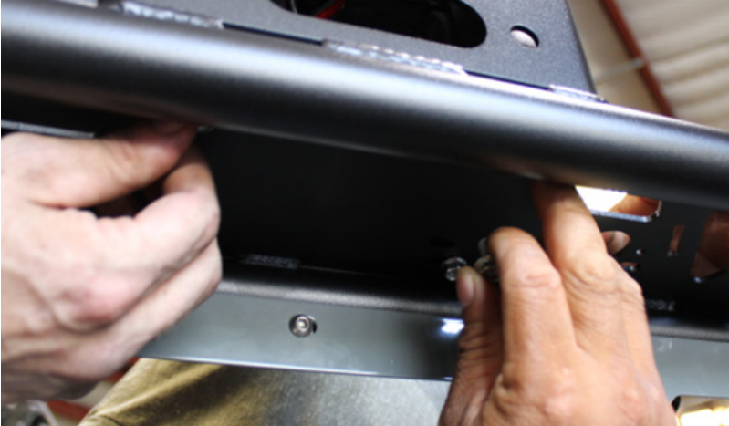
FIG 5 - Fasten Winch to Winch Mount Plate using 10mm Socket
