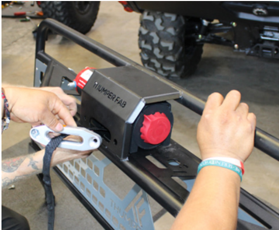
FIG 3 - Thread Winch Cable through Fairlead
