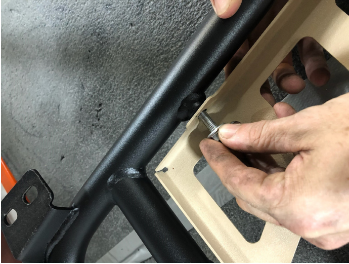
FIG 1 - Fasten Accent Panel to Headache rack using 13 mm socket
