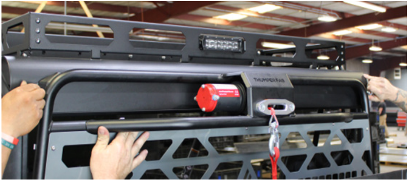
FIG 7 - Loosely fasten Headache Rack top bolts using 13mm Socket
