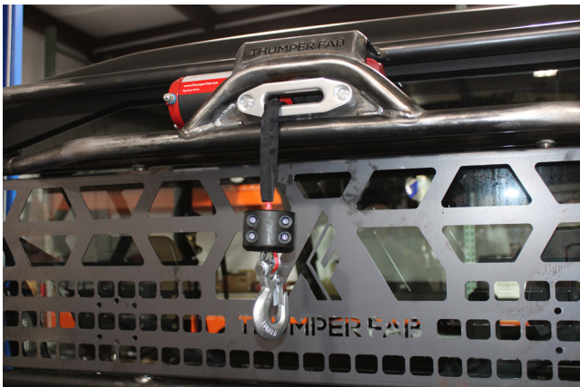
FIG 8 - Fasten Winch Hook And Winch Stop To Winch Cable - 4 mm Allen
