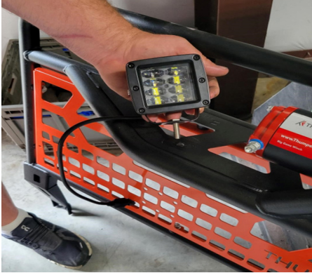
FIG 12 - Fasten Cube Light to Headache Rack
