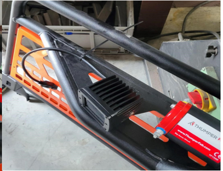
FIG 13 - Ziptie Cube Light Pigtail to Headache Rack
