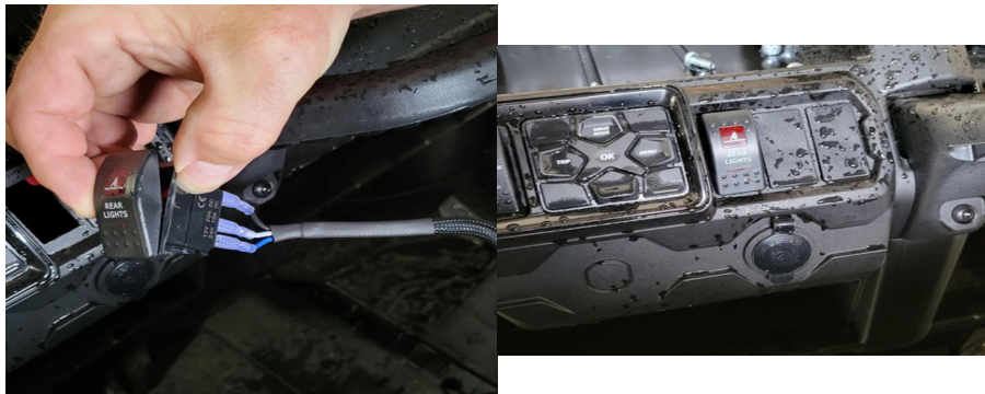
FIG 16 & FIG 17 - Select slot for switch, check wiring before installation. Snap switch into slot in dash.
