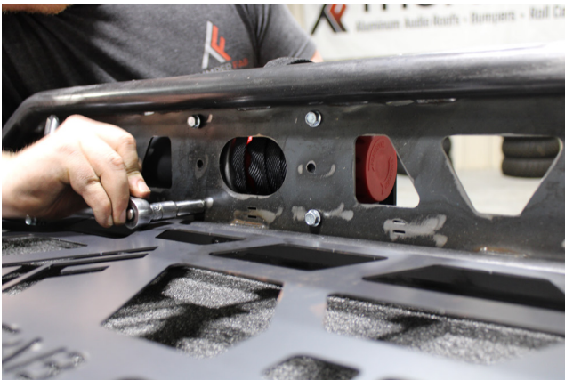
FIG 4 - Fasten Winch To Winch Base Plate - 10 mm Socket
