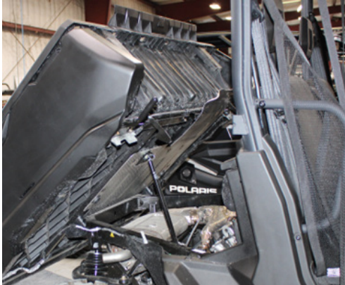
FIG 5 - Raise Dump Bed To Fully Open Position
