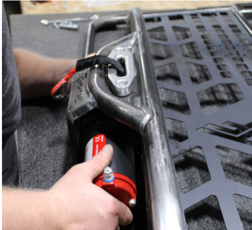
FIG 3 - Thread Winch Cable Through Fairlead
