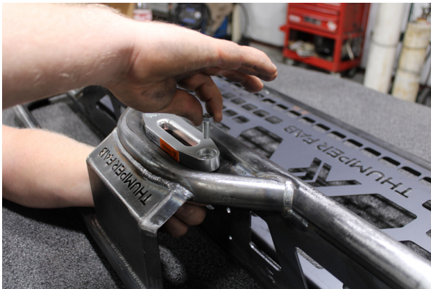
FIG 2 - Fasten Fairlead To Headache Rack - 13 mm Socket & Wrench
