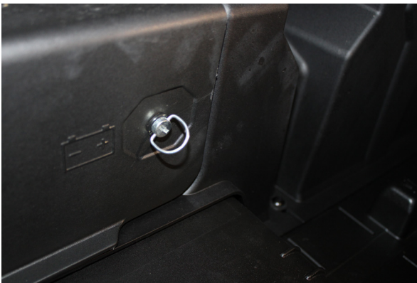
FIG 10 - Remove Twist Release Pins To Gain Access To Battery
