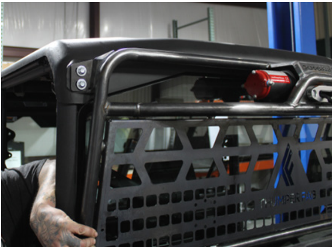
FIG 6 - Loosely Install Upper Bolts
