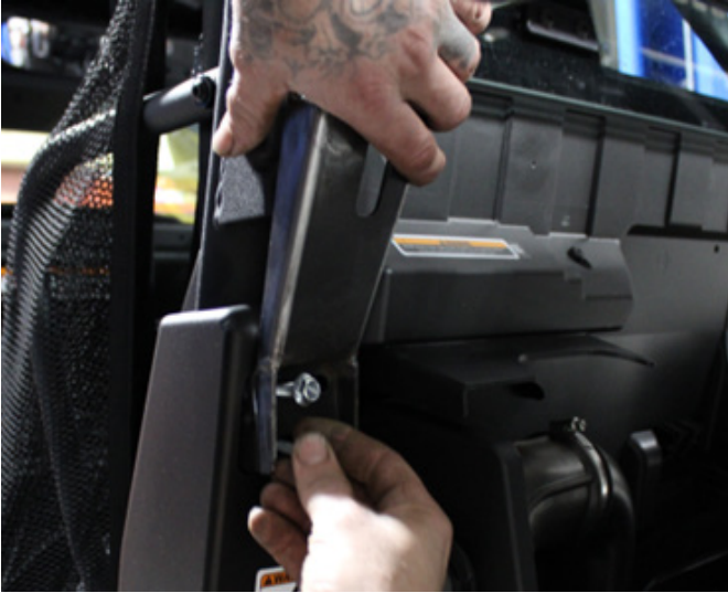
FIG 7 - Fully Tighten Flange Bolts (B) Using 13mm Socket And Ratchet
