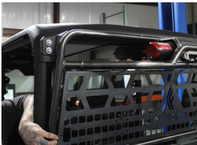
FIG 6 - Loosely Install Upper Bolts
