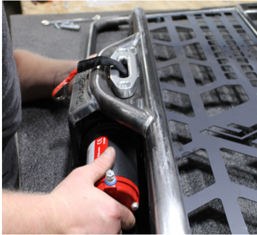
FIG 3 - Thread Winch Cable Through Fairlead
