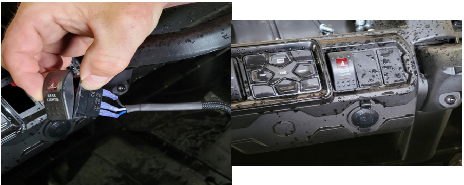
FIG 19 & FIG 20 - Select slot for switch, check wiring before installation. Snap switch into slot in dash.
