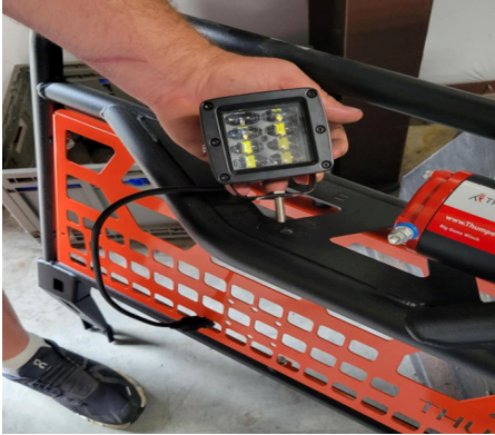
FIG 15 - Fasten Cube Light to Headache Rack
