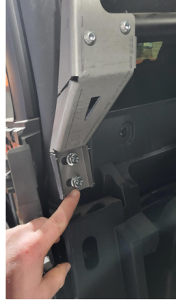
FIG 13 & FIG 14 - Fasten Lower portion of Headache Rack to Vehicle
