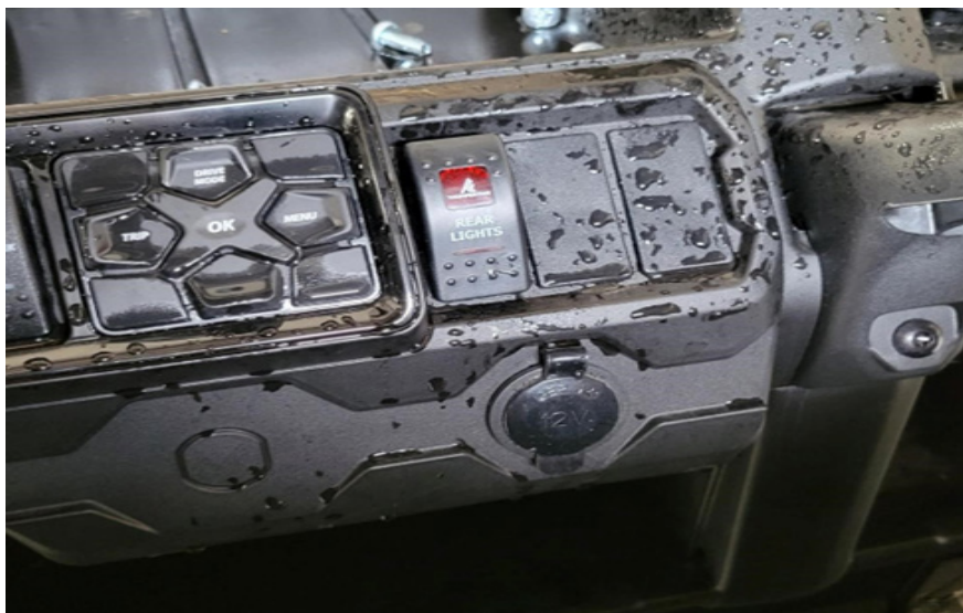
FIG 29 - Install the switch in the dash
