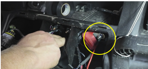
FIG 21 - Connect Winch Wires
