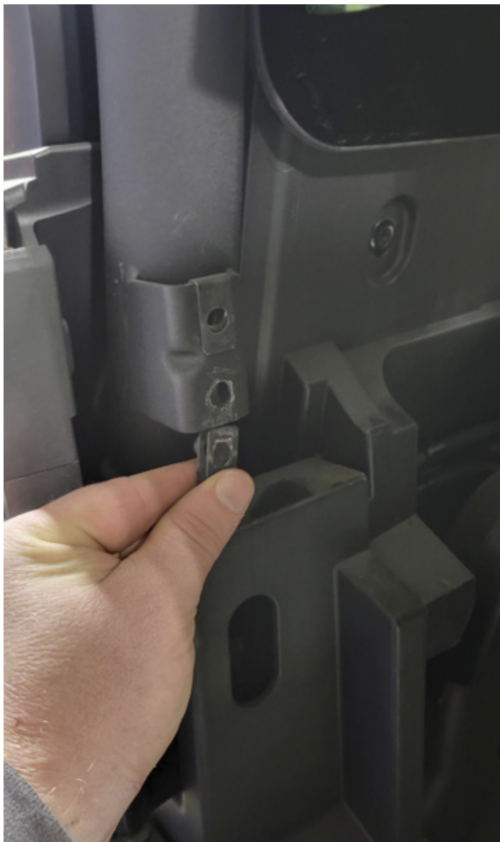
FIG 11 - Install M8 Clip on Barrel Nuts (2020+ Brackets ONLY)
