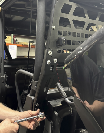
FIG 13 & FIG 14 - Fasten Lower portion of Headache Rack to Vehicle
