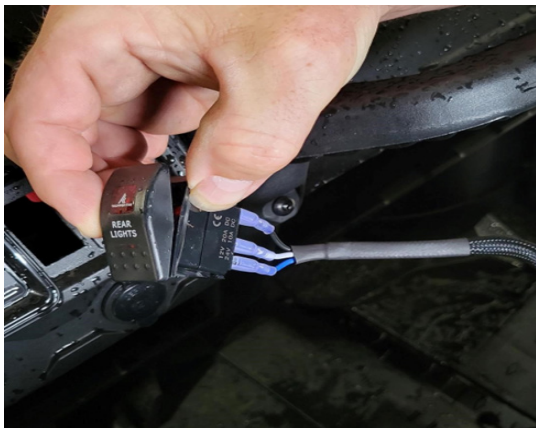
FIG 28 - Connect Wires to Switch
