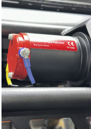
FIG 20 - Connect wires to the Winch
