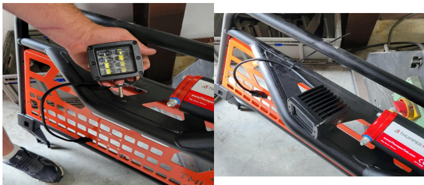
FIG 22 & FIG 23 - Fasten Cube Light to Headache Rack. Zip tie Cube Light wires to Headache rack frame
