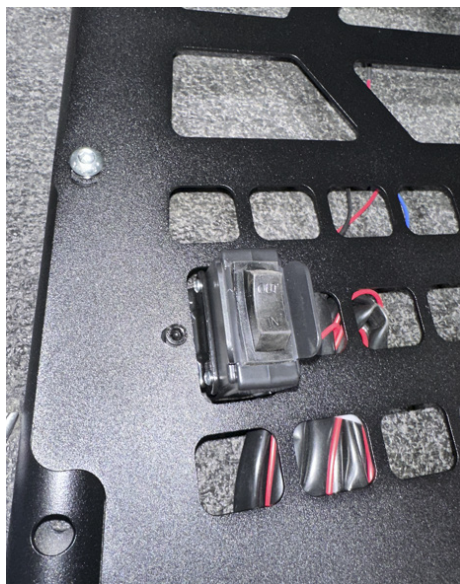
FIG 3 - Fasten Manual Switch to the Rear Panel
