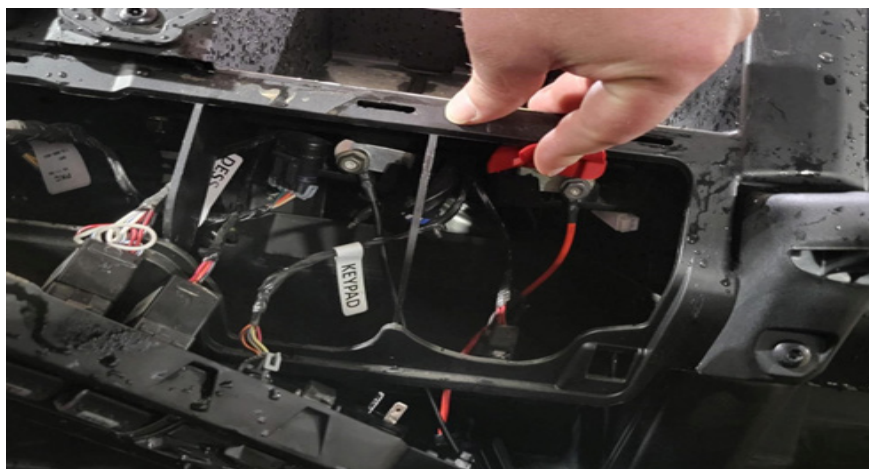
FIG 25 - Connect red wire to red terminal and black wire to black terminal
