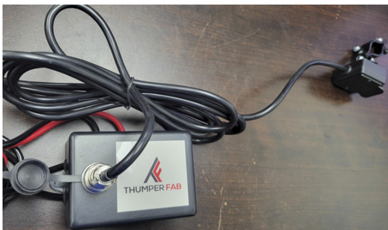
FIG 18 - Tighten switch harness to contactor box
