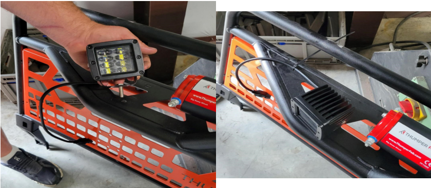
FIG 26 & FIG 27 - Fasten Cube Light to Headache Rack. Zip tie Cube Light wires to Headache rack frame
