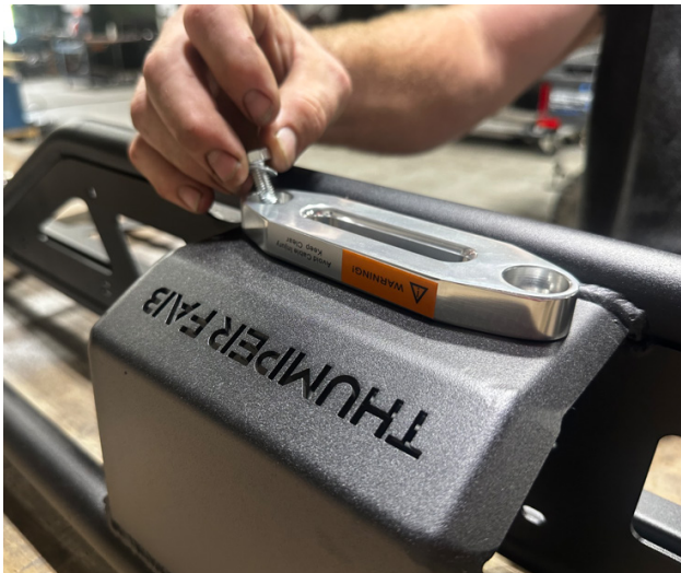
FIG 6 - Fasten Fairlead to the Headache Rack Frame
