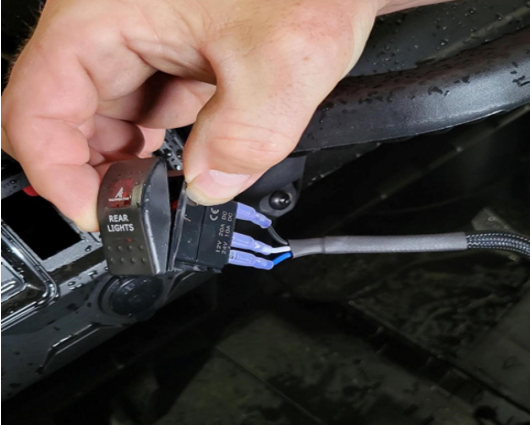
FIG 30 - Connect Wires to Switch
