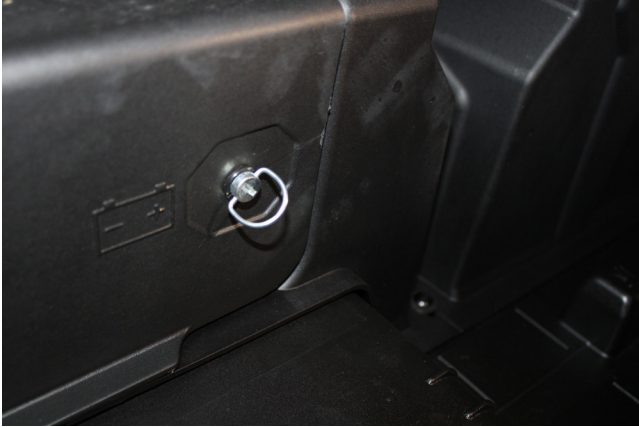
FIG 15 - Remove twist release pins to gain access to the battery
