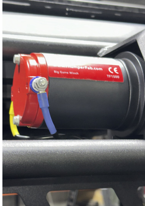
FIG 22 - Connect wires to the Winch
