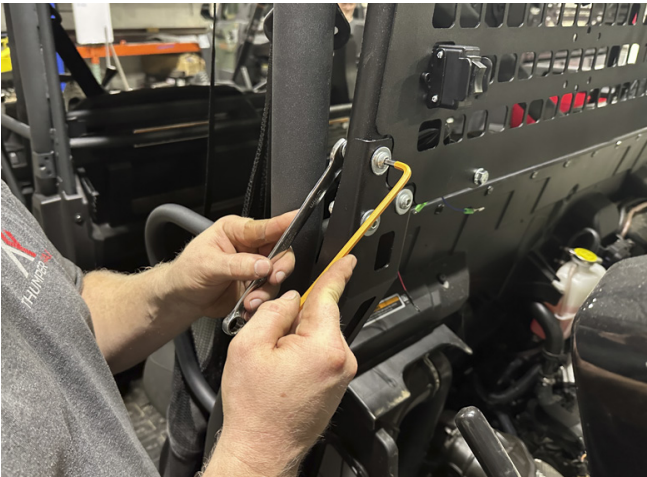
FIG 14 - Tighten Lower Mount Brackets
