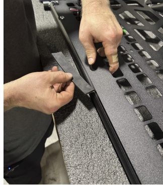
FIG 1 & FIG 2 - Fasten Rear Panel to the Headache Rack Frame
