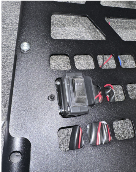
FIG 3 - Fasten Manual Switch to the Rear Panel
