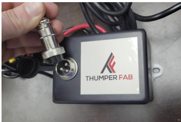
FIG 17 - Plug manual switch harness into winch contactor box
