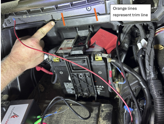
FIG 19 - Grind down plastic lip for Winch Control Box
