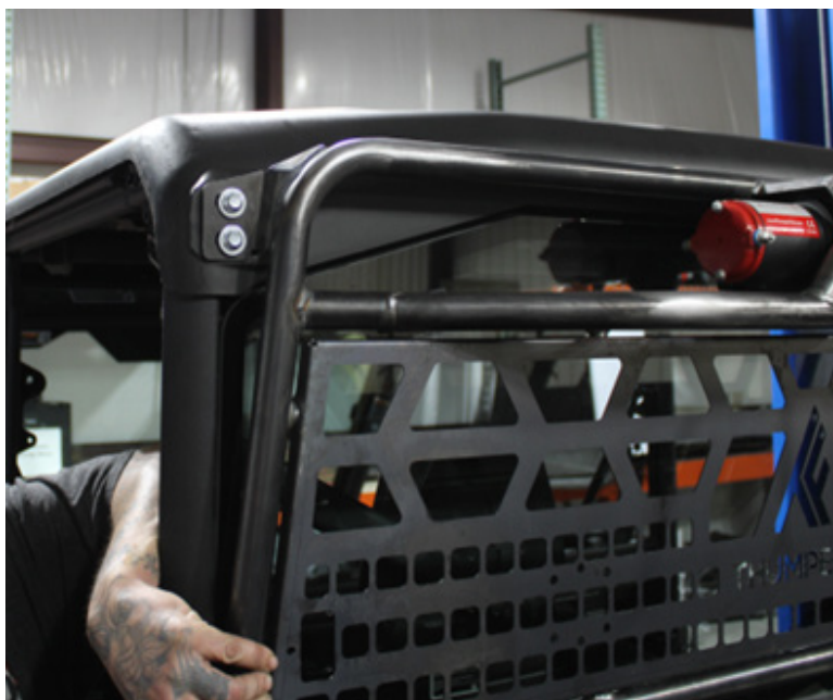
FIG 12 - Fasten Headache Rack to Vehicle
