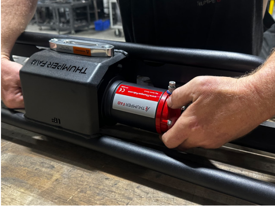
FIG 7 - Fasten Winch to the Headache Rack Frame
