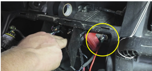
FIG 23 - Connect Winch Wires
