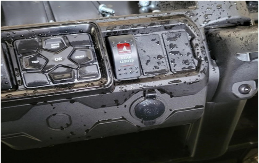
FIG 31 - Install the switch in the dash
