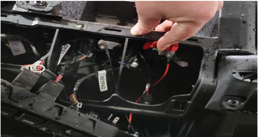
FIG 29 - Connect red wire to red terminal and black wire to black terminal
