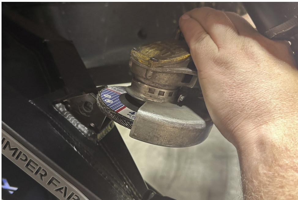
Grind Shock Cradle down to make clearance for shock body
