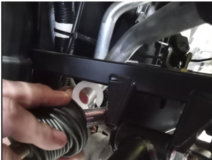
Install 2 x Steering Stops on Worm Gear (On Each Side)
