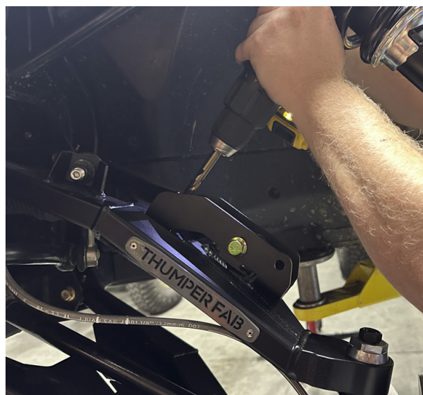
Drill hole through Upper Control Arm using an 13/32" Drill Bit
