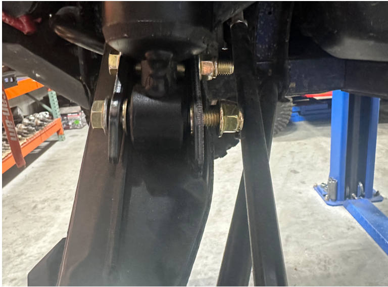
Fasten the shock to the Arm Side Bracket
