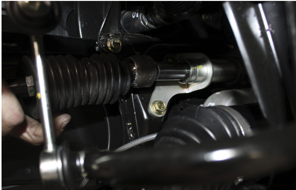
Slide Steering Boot off of Steering Rack
