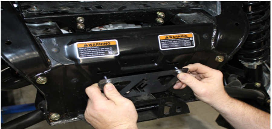
FIG 4 - Install Logo Plate using 10mm Socket and 10mm Wrench
