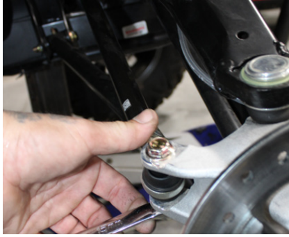
FIG 3 - Remove cotter pin and disconnect tie rod end from hub assembly using 15mm Socket and 15mm Wrench
