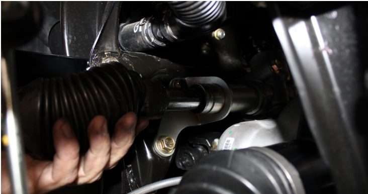
FIG 16 - Slide steering boot back to gain access to worm gear
