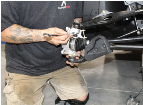
FIG 5 - Disconnect upper ball joint using 18mm Wrench
