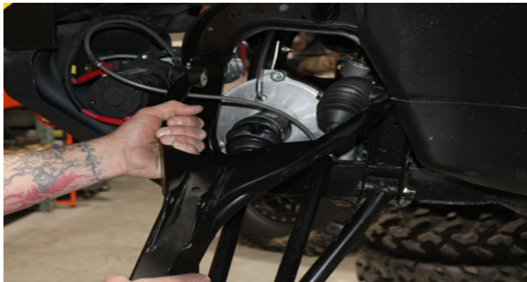
FIG 7 - Remove Upper Control Arm using 15mm Socket and 15mm Wrench
