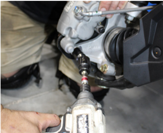
FIG 2 - Remove the Brake Caliper
