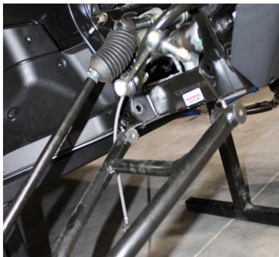
FIG 8 - Remove Lower Control Arm using 15mm Socket and 15mm Wrench
