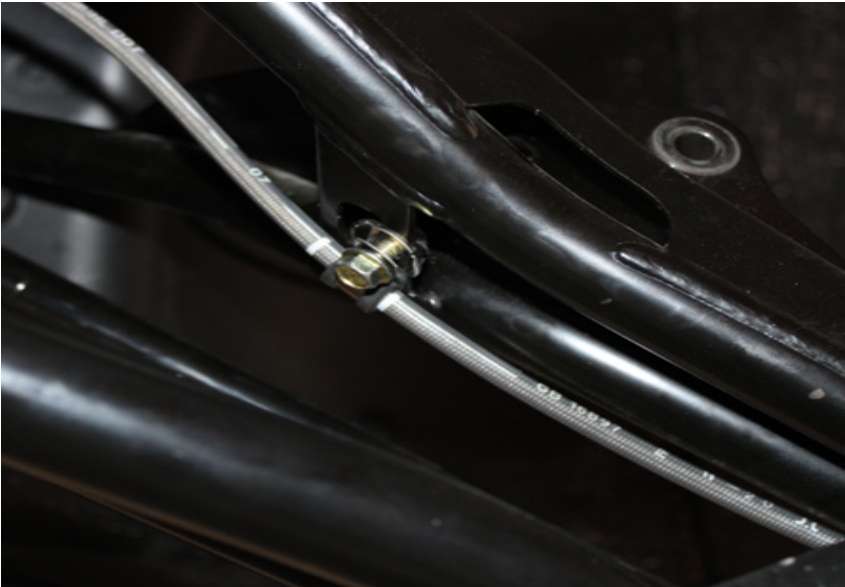
FIG 4 - Disconnect the brake line from the underside of upper control arm using 10mm socket
