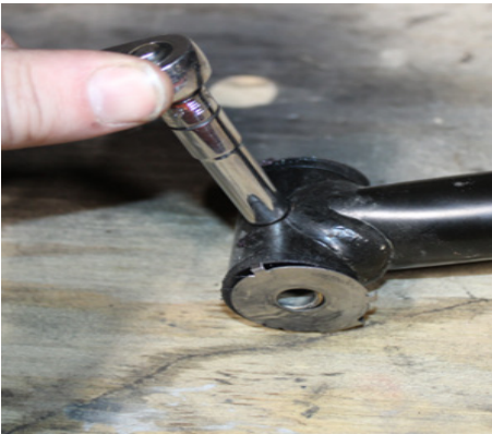
FIG 9 - Install OEM grease fittings into Thumper Fab arms using 7mm Socket
