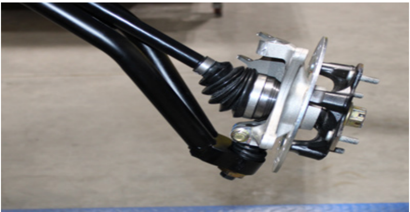
FIG 11 - Fasten knuckle to lower ball joint using 15mm Socket and 15mm Wrench
