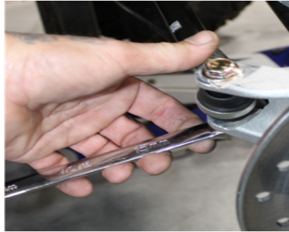
FIG 18 - Fasten tie rod to knuckle using OEM bolt and nut including new cotter pin. Adjust toe as needed
