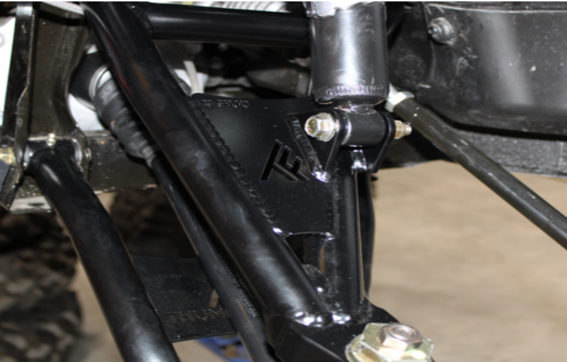
FIG 13 - Fasten shock to upper control arm using 15mm Wrench and 15mm Socket
