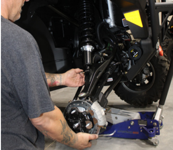
FIG 1 - Remove Wheels, Axle Nuts, and Shock lower mounting bolt
