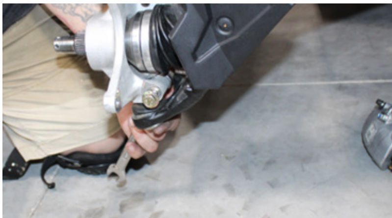
FIG 6 - Disconnect lower ball joint from knuckle using 15mm Wrench and 15mm Socket
