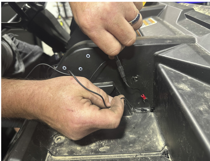
FIG 4 - Feed Terminal end of Wiring Harness (2) through hole
