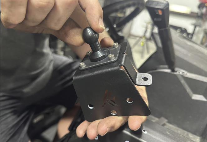
FIG 5 - Mount Ball Mount to Mount Bracket using 9/64" Allen and 11/32" Wrench
