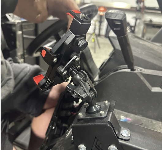
FIG 7 - Mount the Phone Charging Unit (3) to the Ball Mount (4) using the Adjustable Swivel Mount (5)
