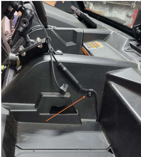
FIG 8 - Connect pigtail from Phone Charging Unit (3) to the Wire Harness (2)
