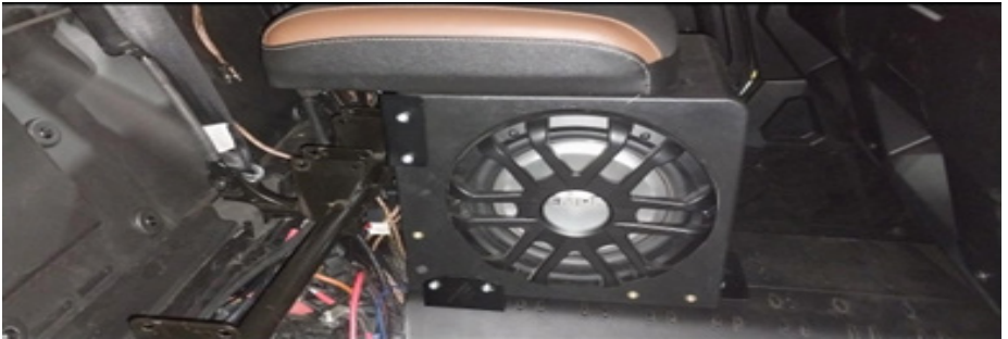
FIG 6 - Mount Brackets to Subwoofer using a T30 Torx
