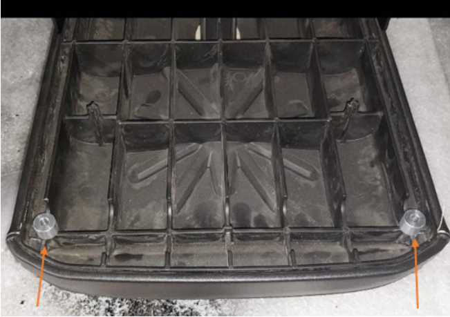
FIG 3 - Place Spacers on underside of seat
