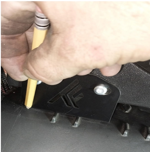
FIG 7 - Mark position of Lower Bracket using a Pencil or Marker
