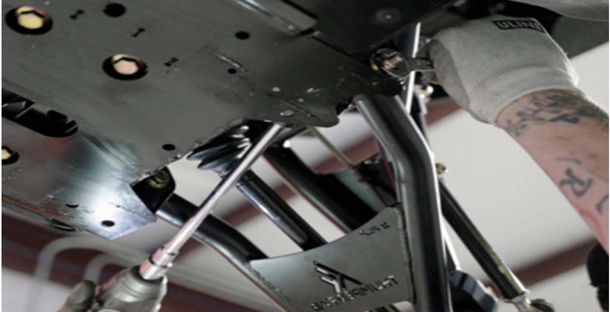
FIG 1 - Remove Lower Control Arm mounting bolts using 15mm Socket and 15mm Wrench
