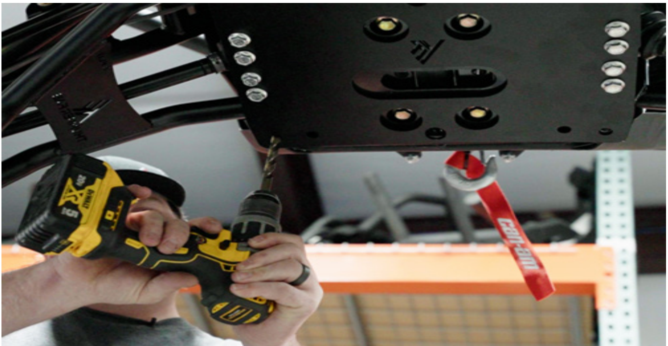
FIG 6 - Use 13/32" Drill bit to enlarge OEM holes in frame using Main Plate as a template
