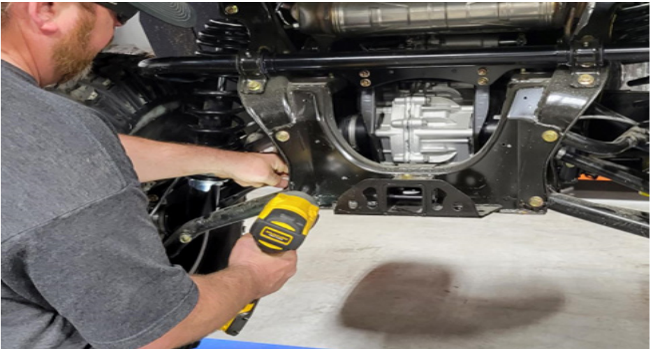
FIG 2 - Use 15mm Socket and 15mm Wrench to remove OEM bolts
