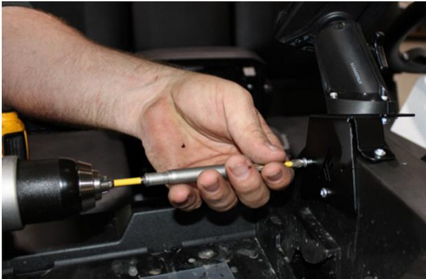
**FIG 2 - Fasten Dash Mount Plate to dash using Drill**
