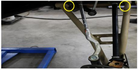
FIG 6 - Remove Lower Control Arm using 15mm Socket, 18mm Socket and 18mm Wrench Install Polaris General Steering Stop
