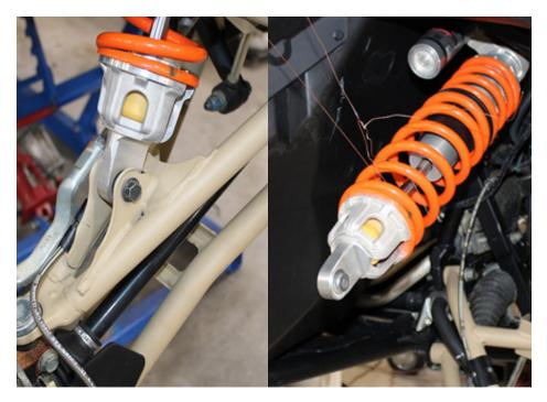
FIG 1 - Remove Shock Bolt using 15mm Socket and 15mm Wrench
