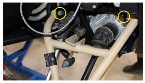
FIG 5 - Remove the Upper Control Arm using the 18mm Socket and the 18mm Wrench
