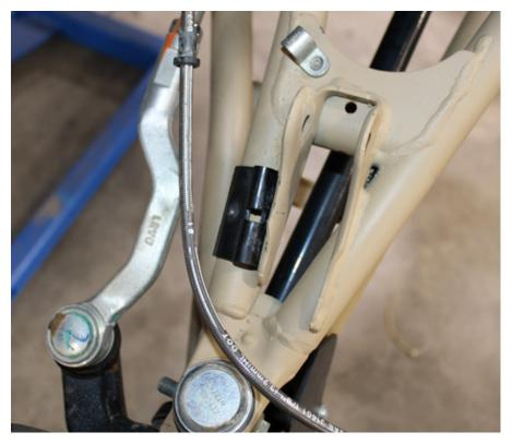
FIG 3 - Unfasten Brake Line from Control Arm using Flat Head Screwdriver
