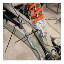
FIG 10 - Use provided Zip Ties to fasten Brake Line to Upper Control Arm
