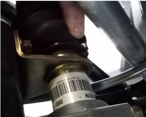
**FIG 8 - Locate and cut Zip Tie using Snips**
