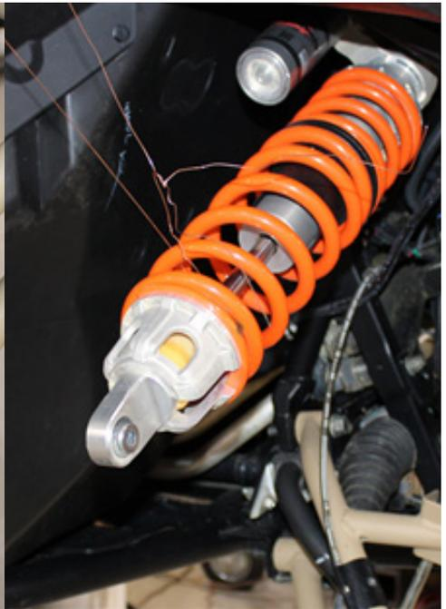
**FIG 2 - Tie Shock out of the way for Control Arm Removal and Replacement**
