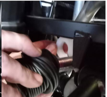
**FIG 9 - Press Steering Stop (B) onto Worm Gear Shaft**
