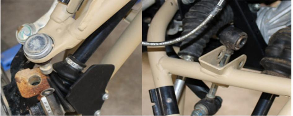
**FIG 4 - Unfasten the Upper Ball Joint and the Sway Bar Link using the 15mm Socket and 15mm Wrench**
