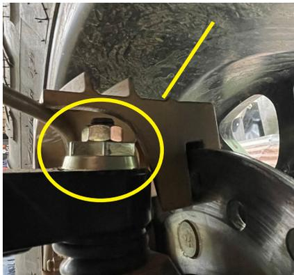
**FYI - Stock Ball Joints are Compatible with Rock Guard, Trim or Remove Rock Guard if Running Keller or Uniball Ball Joints**
