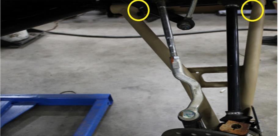
**FIG 6 - Remove Lower Control Arm using 15mm Socket, 18mm Socket and 18mm Wrench**
