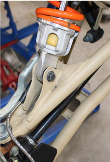
**FIG 1 - Remove Shock Bolt using 15mm Socket and 15mm Wrench**
