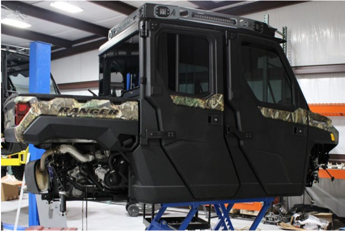
FIG 1 - Prepare Ranger by Removing Parts to Access Arms
