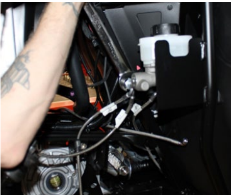
FIG 9 - Remove Factory Brake Lines
