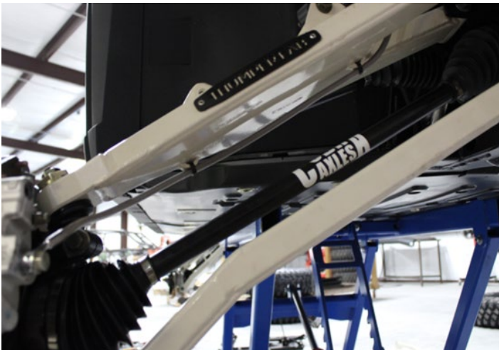
FIG 12 - Mount Brake Rotor and Caliper using factory hardware. Fasten Brake Line to upper arm using Zip Ties
