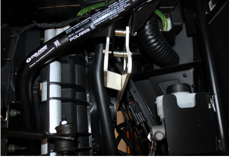
FIG 33 - Install OEM Shock Relocation Brackets - Inner and Outer using 15mm Socket and 15mm Wrench
