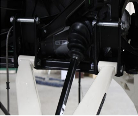
FIG 22 - Slide axle into Rear Differential
