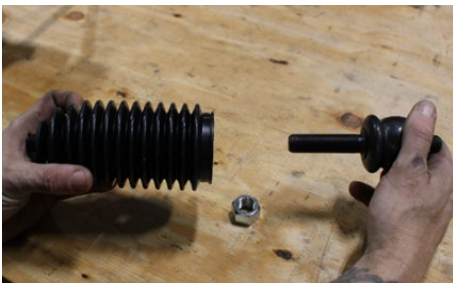
FIG 6 - Slide Steering Boot over Inner Tie Rod
