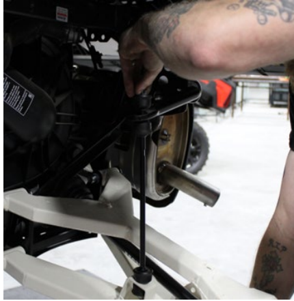
FIG 25 - Fasten Sway Bar Link to Sway Bar
