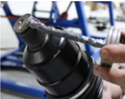
FIG 2 - Use Anti-Seize on Axles
