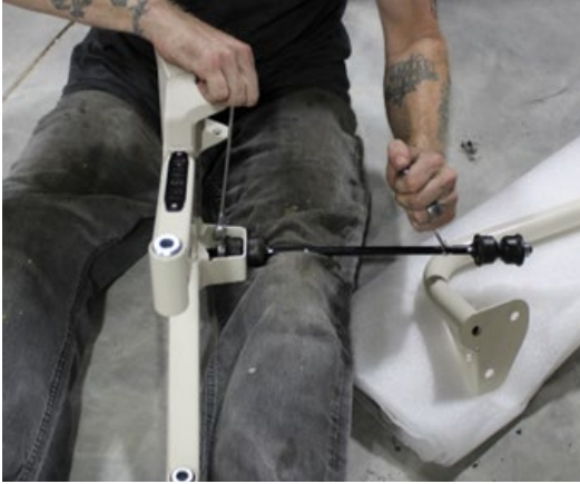
FIG 20 - Fasten Outer Tie Rod to Knuckle
