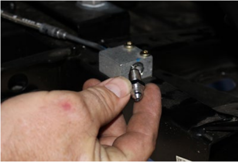
FIG 28 - Install Brake Line Adapter Fittings using 12mm Wrench
