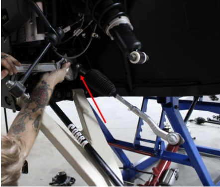
FIG 4 - Remove Factory Tie Rod
