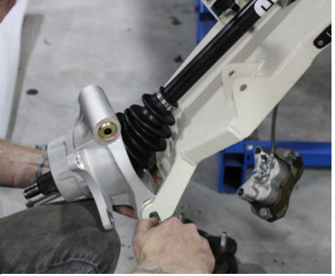
FIG 23 - Loosely mount Rear Knuckle
