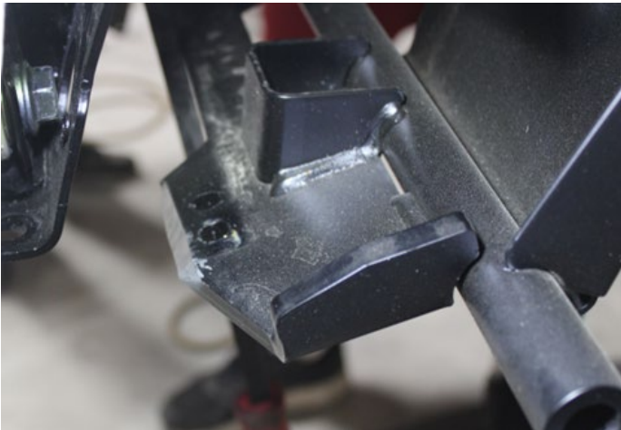
FIG 19 - Use Grinder to clearance Front Bumper
