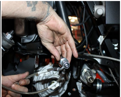
FIG 10 - Install New Brake Lines
