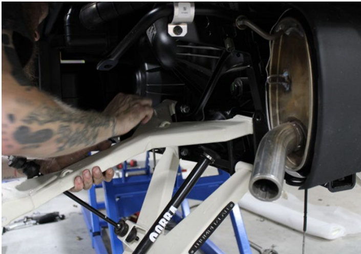
FIG 24 - Install Upper Control Arm using 19mm Socket and 19mm Wrench
