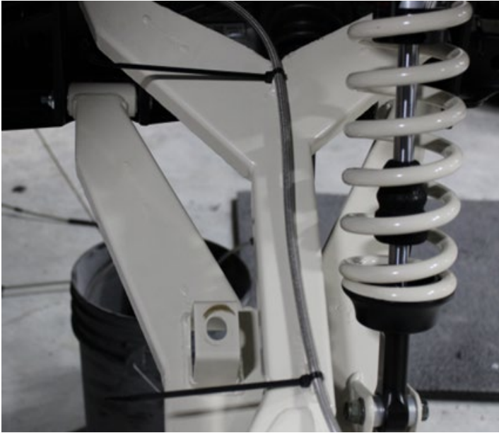
FIG 32 - Fasten brake lines to Upper Control Arm using Zip Ties
