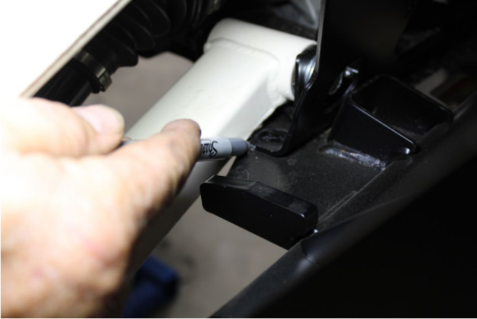
FIG 18 - Mark Front Bumper for Clearancing with Grinder
