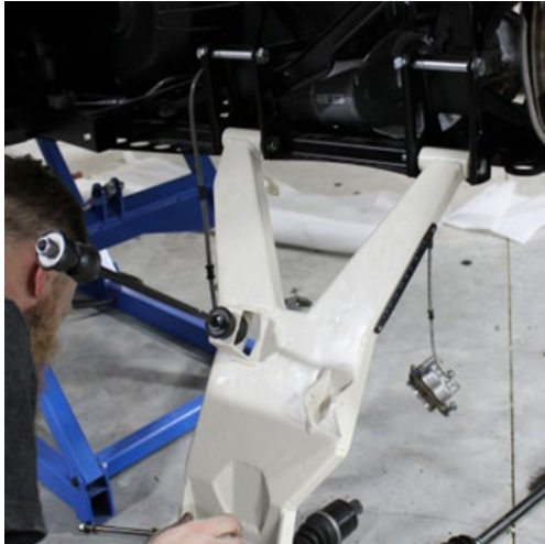
FIG 21 - Attach Lower Control Arm to Frame
