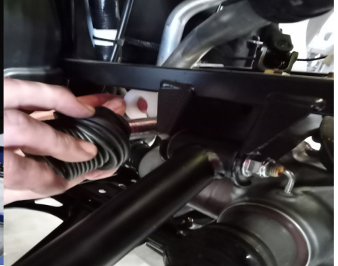
FIG 5 - Install Polaris Steering Stop onto Worm Gear Shaft (OPTIONAL)
