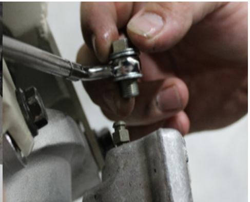
FIG 31 - Fasten Caliper end of Brake line using 13mm Socket using Factory Bolt and Hardware
