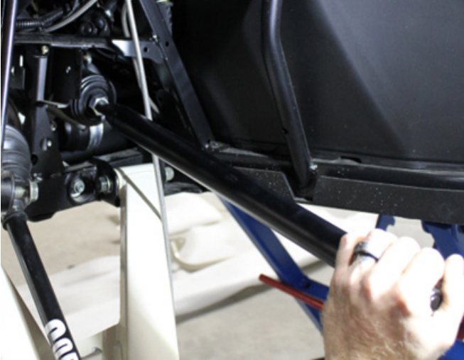
FIG 8 - Install Tie Rod Main Body onto Inner Tie Rod
