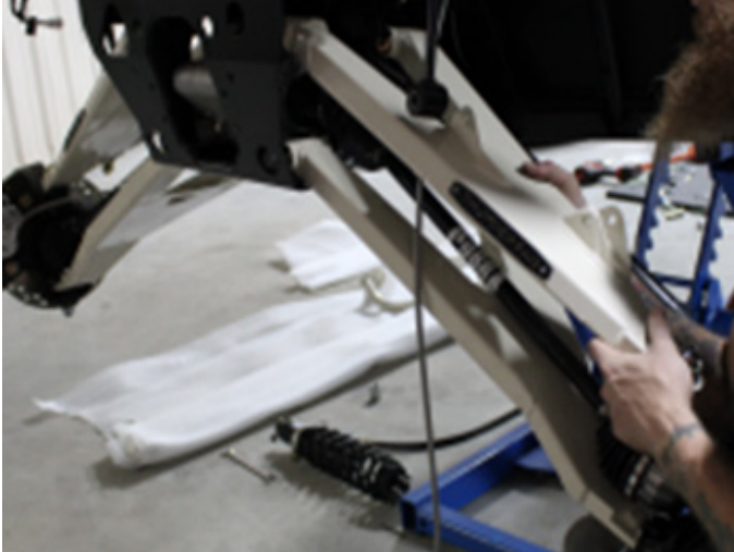
FIG 11 - Install Upper Control Arm using 18mm Socket and 18mm Wrench
