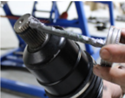
FIG 2 - Use Anti-Seize on Axles
