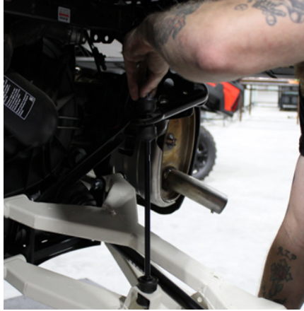
FIG 25 - Fasten Sway Bar Link to Sway Bar
