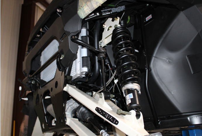
FIG 35 - Install OEM Shock using factory hardware and tighten with 15mm Socket and 15mm Wrench
