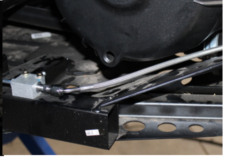
FIG 29 - Install Rear Brake Lines using 11mm Wrench
