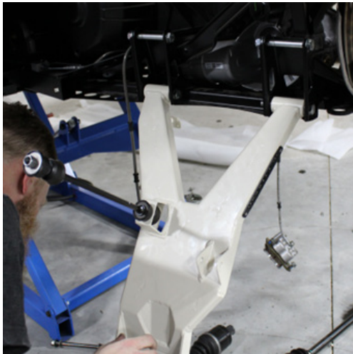
FIG 21 - Attach Lower Control Arm to Frame
