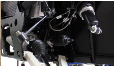
FIG 7 - Tighten Inner Tie Rod to Steering Rack Using Crescent Wrench
