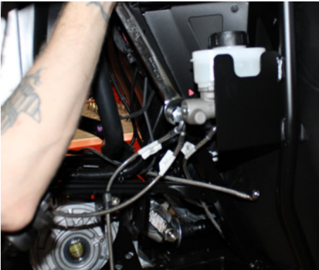
FIG 9 - Remove Factory Brake Lines
