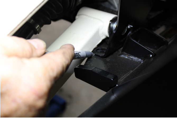
FIG 18 - Mark Front Bumper for Clearancing with Grinder
