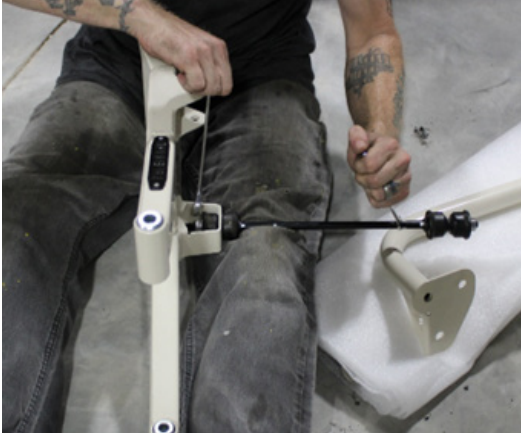
FIG 20 - Fasten Outer Tie Rod to Knuckle
