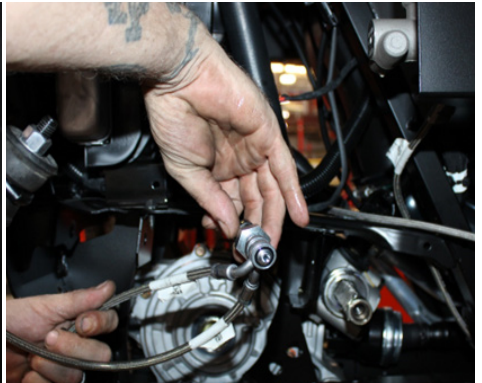
FIG 10 - Install New Brake Lines
