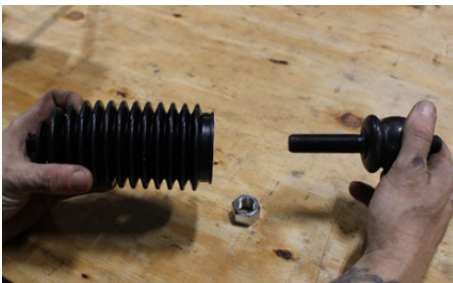
FIG 6 - Slide Steering Boot over Inner Tie Rod
