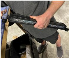
Next, place the 6 inch light bars (2) into the rear rail and both of the 20 inch light bars into the side rails as shown below. Use more of the 1/4"-20 hardware in the kit.
