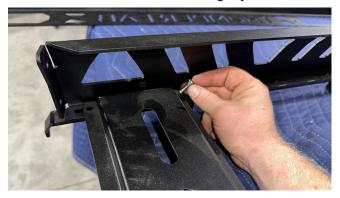
Next, start fastening the front and rear rails onto the upper roof rack with more of the provided 1/4"-20 hardware, as shown below.
