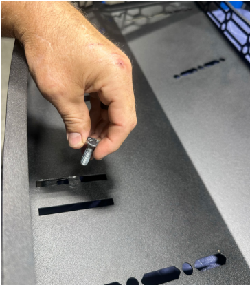
FIG 11 & FIG 12 - Fasten Bumper Mount Brackets to Main Basket
