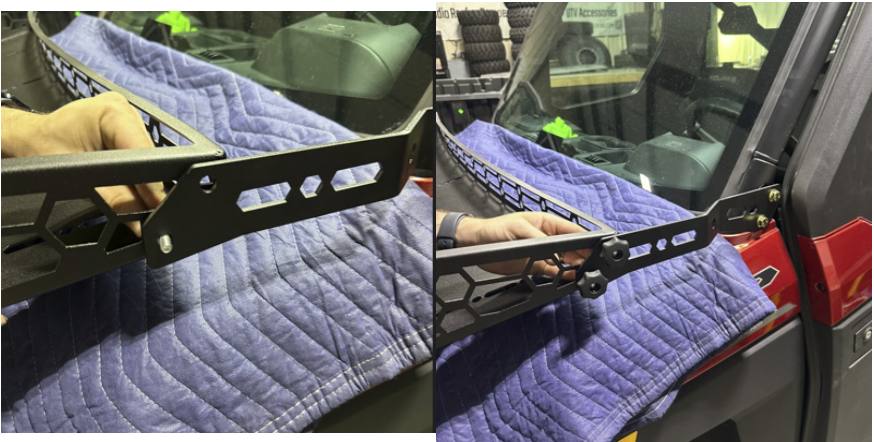
FIG 6 & FIG 7 - Mount Basket to Rear Mount Brackets
