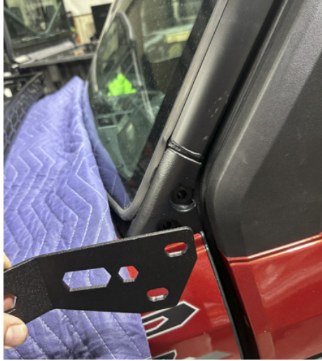
FIG 3 - Remove 4 x A Pillar cage bolts, save nylon lock nuts
