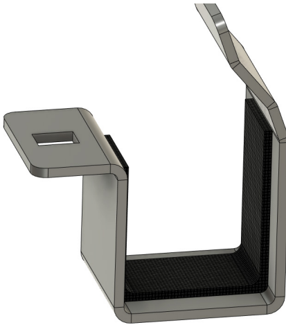
FIG 18 - Apply foam to Lower Bull Bar Mounts
