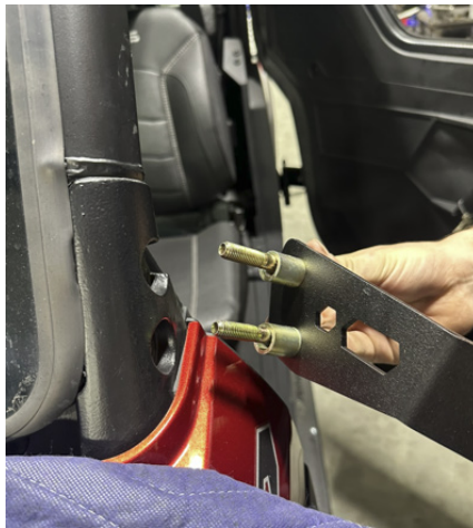
FIG 4 - Prepare Mount Brackets for installation
