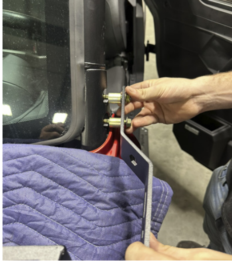
FIG 5 - Fasten rear mount brackets to vehicle
