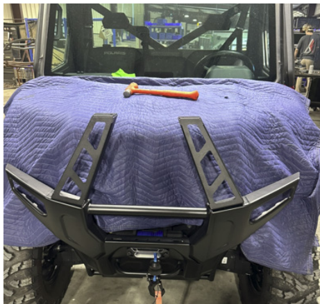
FIG 1 & FIG 2 - Loosely mount bumper mount brackets using a 13mm socket and wrench
