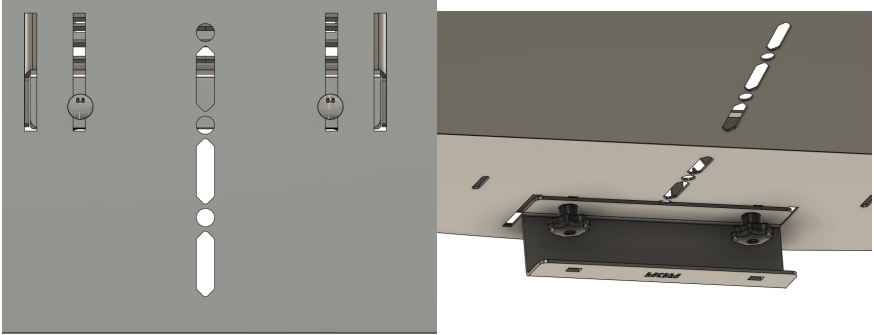
FIG 14 & FIG 15 - Fasten Upper Bull Bar mount to Main Basket
