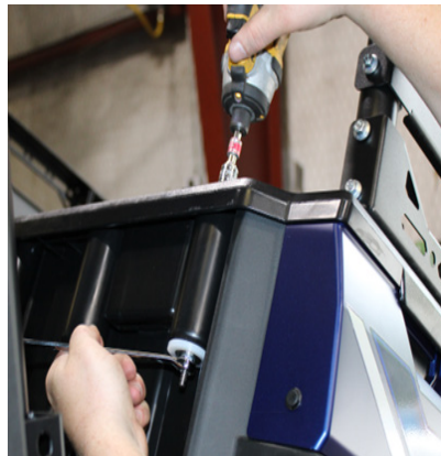
FIG 5 - Using 7/16" Socket & 7/16" Wrench Install Plastic Retainers to Front Corners of Bed
