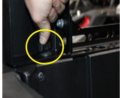
FIG 4 - Insert Kolpin Lock & Ride Mounts in Corners of Bed. Lift Bed once Mounts have been Tightened
