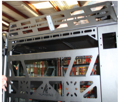
FIG 17 - Fasten together Upper Rack - FRONT and Upper Rack - REAR using 10mm Socket and 10mm Wrench
