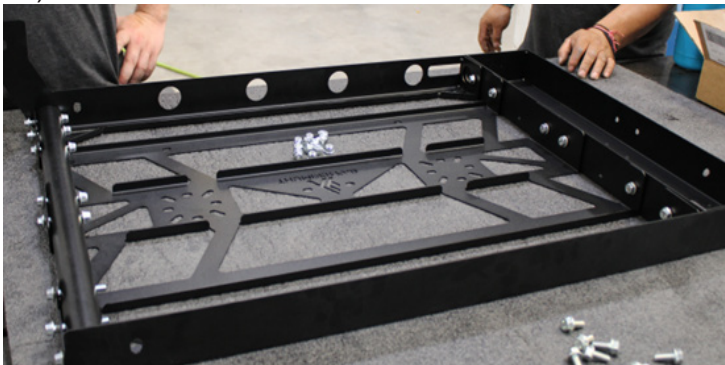
FIG 2 - Hand Tighten Hardware for Each Side
