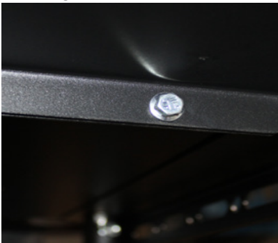
FIG 17 - Fasten together Upper Rack - FRONT and Upper Rack - REAR using 10mm Socket and 10mm Wrench
