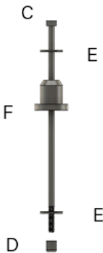
FIG 5 - Using 7/16" Socket & 7/16" Wrench Install Plastic Retainers to Front Corners of Bed
