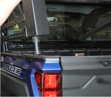
FIG 4 - Insert Kolpin Lock & Ride Mounts in Corners of Bed. Lift Bed once Mounts have been Tightened
