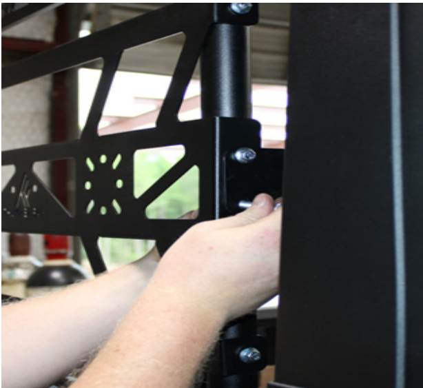
FIG 7 - Connect the Rear Brace to the Bed Rack using a 13mm Socket and 13mm Wrench
