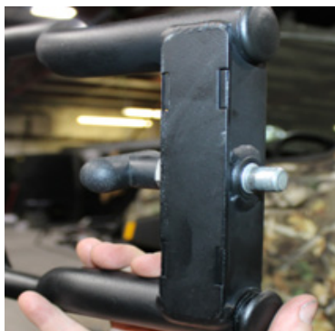
FIG 21 - Install Plastic Tubing Plugs (O)
