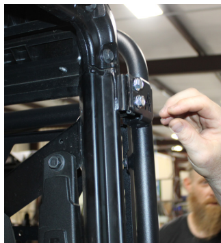
FIG 6 - Fasten Headache Rack Bolts using 13mm Socket
