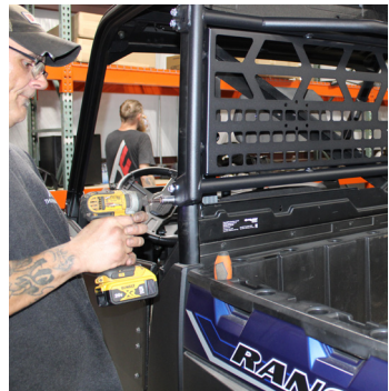
FIG 6 - Fasten Headache Rack Bolts using 13mm Socket
