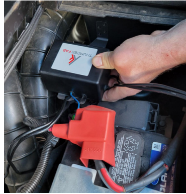
FIG 8 - Fasten winch contactor to inside of battery box using supplied bracket
