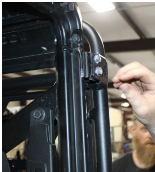
FIG 6 - Fasten Headache Rack Bolts using 13mm Socket
