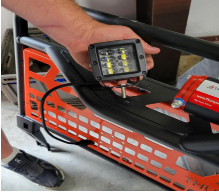
FIG 11 - Fasten cube light to Headache Rack
