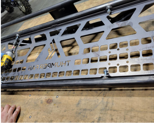
Fig 1 - Install Accent Panel onto Headache Rack with 13mm Socket
