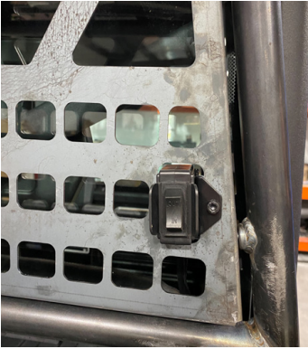
FIG 7 - Fasten switch to accent panel
