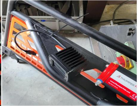
FIG 12 - Zip Tie Cube Light wire pigtail to Headache Rack
