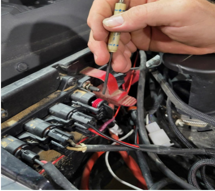
FIG 15 - Remove unused Pulse Bar Plug
