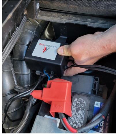
FIG 9 - Fasten winch contactor to inside of battery box using supplied bracket
