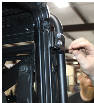
FIG 6 - Fasten Headache Rack Bolts using 13mm Socket
