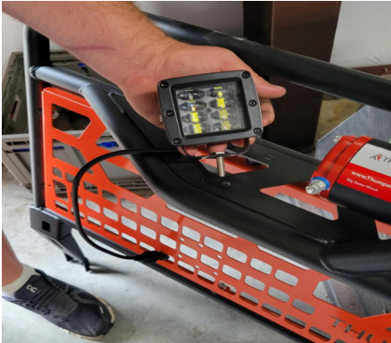
FIG 12 - Fasten cube light to Headache Rack
