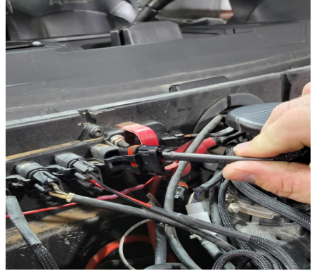
FIG 16 - Plug in Thumper Fab pulse bar pigtail
