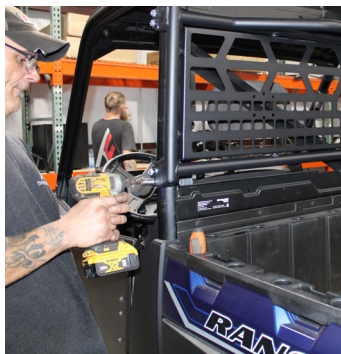
FIG 6 - Fasten Headache Rack Bolts using 13mm Socket
