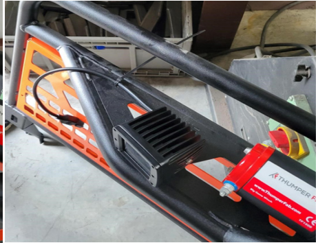
FIG 13 - Zip Tie Cube Light wire pigtail to Headache Rack
