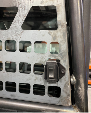
FIG 8 - Fasten switch to accent panel
