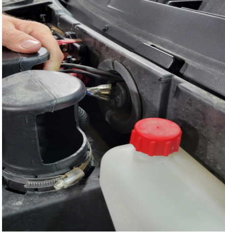
FIG 20 - Feed switch terminals through grommet in firewall
