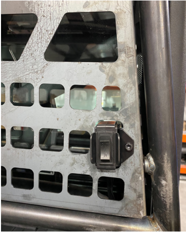
FIG 10 - Fasten switch to accent panel
