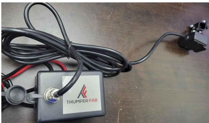
FIG 9 - Tighten switch harness to contactor box
