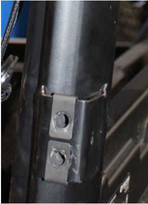
FIG 5 - Install clips on lower brackets, install clips and spacers on the upper if you do not have full doors
