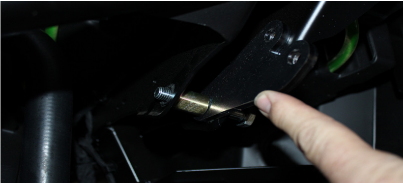
FIG 5 - Install Front Lift Bracket lower Bolt
