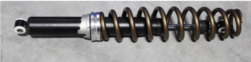
FIG 3 - Install Spring Spacer and Reinstall Spring and Retaining Clip
