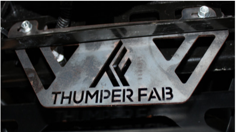
FIG 17 - Fasten logo plate to Rear Bed Frame using 10mm Socket and 10mm Wrench
