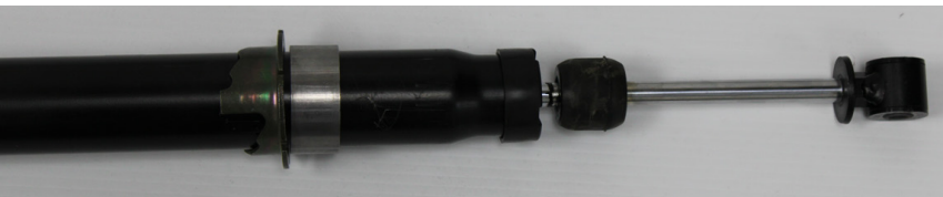
FIG 3 - Install Spring Spacer and Reinstall Spring and Retaining Clip
