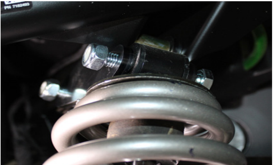
FIG 8 - Reinstall Upper Shock Mount and tighten Flange Bolts (A) using 15mm Socket and 15mm Wrench
