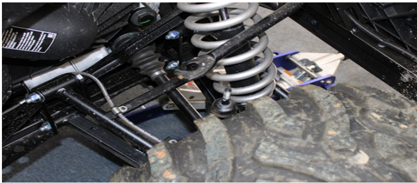
FIG 11 - Remove Rear Sway Bar Hex Nuts using 15mm Socket
