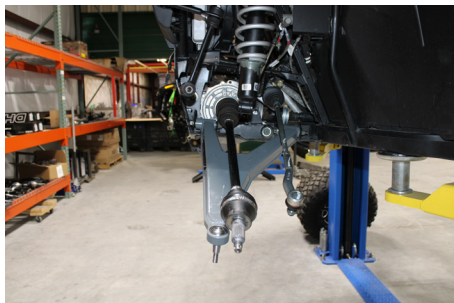
FIG 2 - Mount Lower Control Arms using factory hardware
