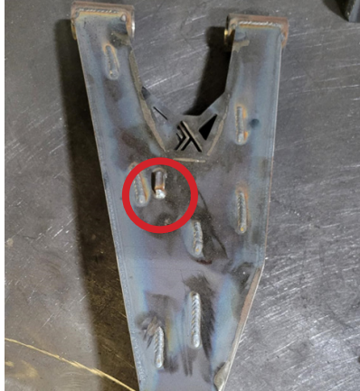
FIG 13 - Zip Tie brake lines to underside of upper control arm
