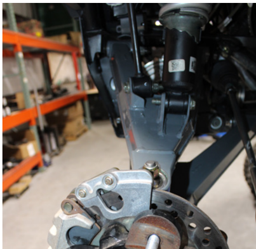
FIG 9 - Fasten sway bar and shock to upper arm using factory hardware and 15mm Socket
