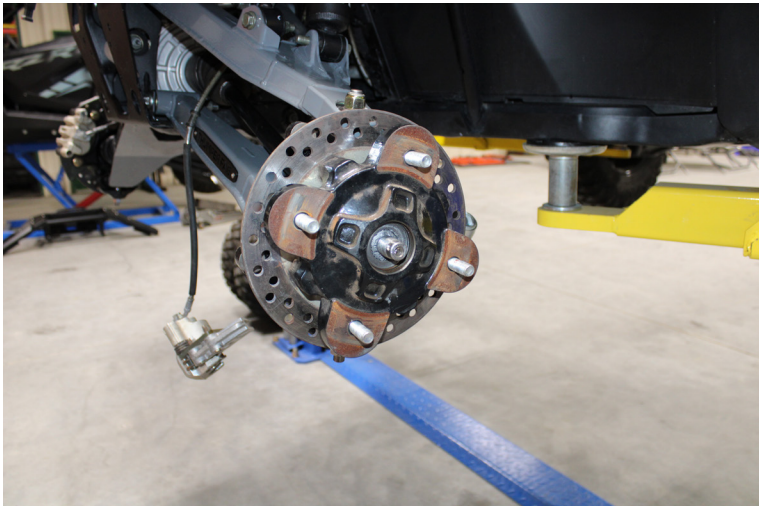
FIG 7 - Slide hub assembly over axle after removing axle nut with 27mm Socket
