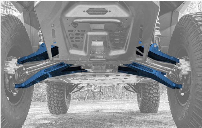
FIG 16 - Lower vehicle and adjust toe as needed
