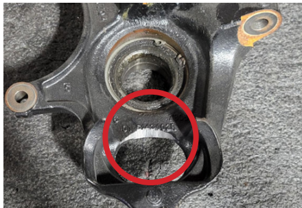
FIG 3 - Clearance knuckle for lower uniball pin
