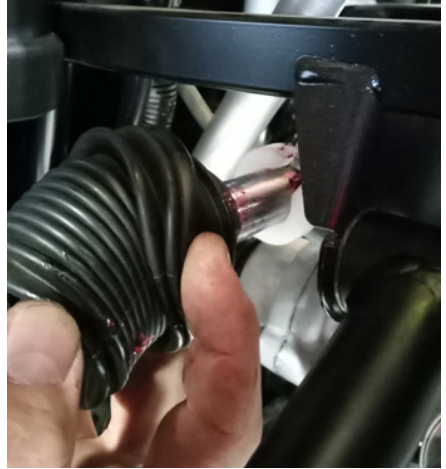
FIG 11 - Slide steering stop onto worm gear
