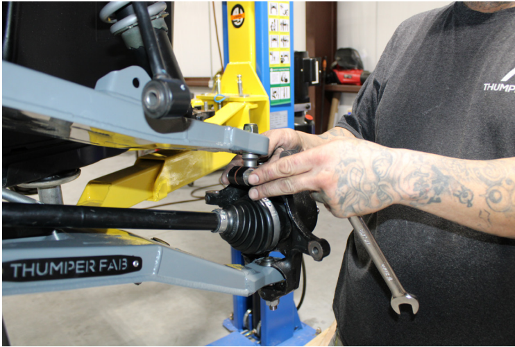
FIG 6 - Tighter pper uniball pin to knuckle using factory cross bolt
