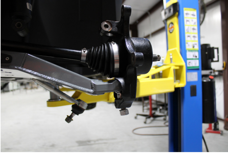
FIG 4 - Tighter Lower uniball pin to Knuckle
