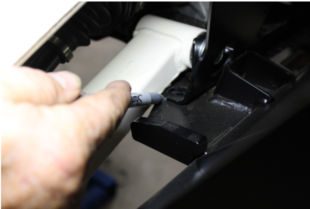
FIG 14 - Mark front bumper for clearancing with grinder
