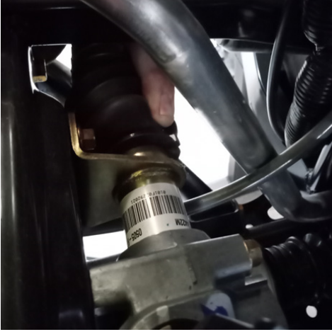
FIG 10 - Cut clamp and slide Boot back
