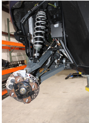
FIG 12 - Fasten tie rod to knuckle using 18mm Socket
